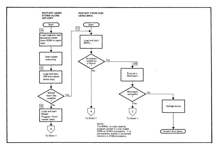
Figure 4-1. Operating Procedures Overview, Flow Diagram (Sheet 2 of 2)
