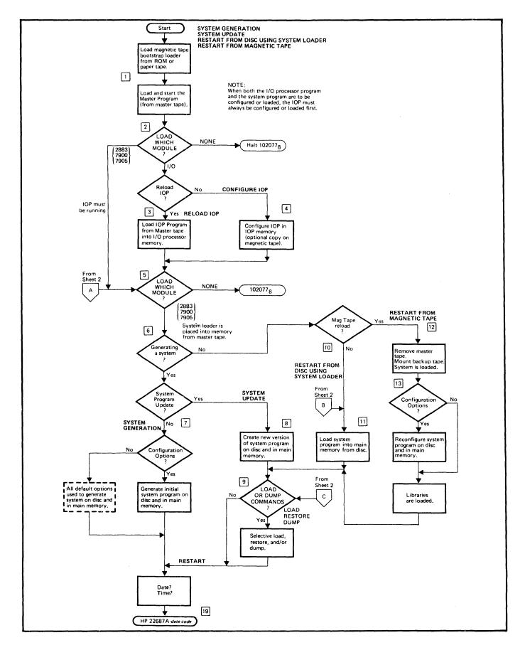
Figure 4-1. Operating Procedures Overview, Flow Diagram (Sheet 1 of 2)
