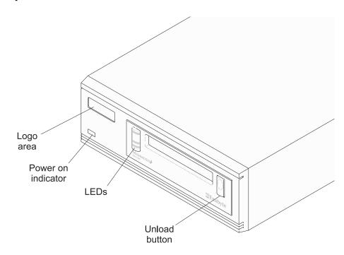
Figure A-3 Front panel components on the tabletop tape drive
