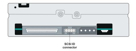
Figure 2-2 Wide SCSI: SCSI ID connector location
