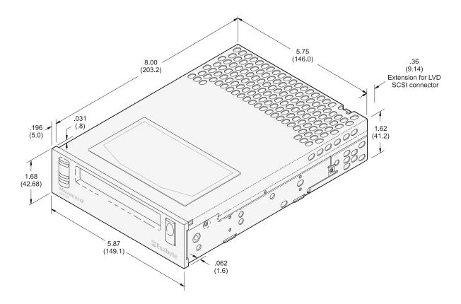
Figure 1-2 Dimensions of the tape drive in inches (and millimeters)
