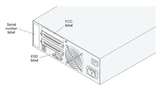
Figure A-5 Label locations for the tabletop model
