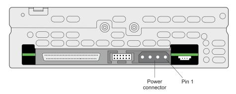
Figure 2-7 Power connector location (LVD wide)
