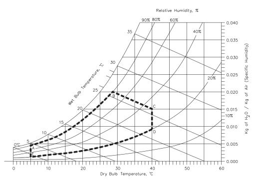
**Figure A-8** Ambient operating environment for the tabletop tape drive
