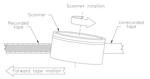
Figure 4-3 Helical-scan recording
