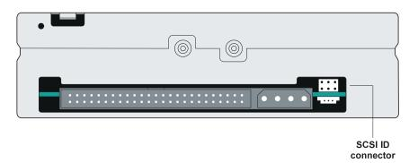
Figure 2-1 Narrow SCSI: SCSI ID connector location
