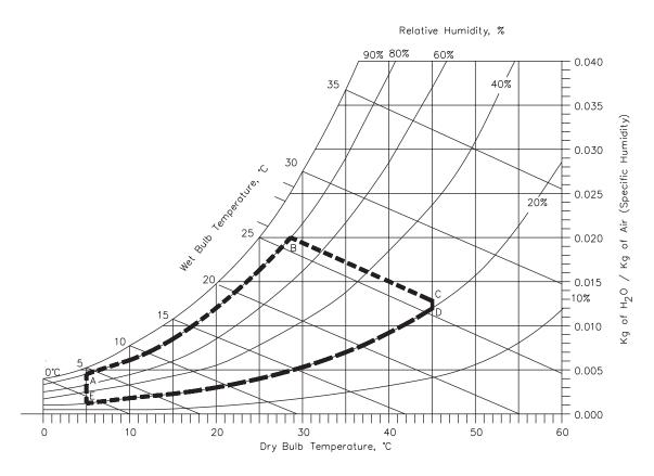
Figure 5-1 Tape path temperature and humidity ranges for operation
