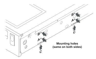
Figure 2-3 Mounting holes
