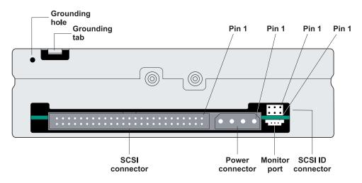
Figure 1-4 Narrow SCSI: back-panel components
