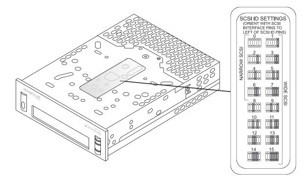
Figure 1-8 SCSI ID label location for the internal model
