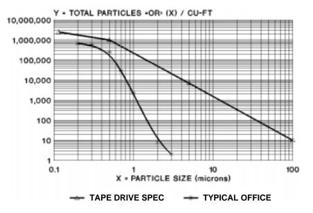
Figure 5-2 Particulate contamination specification vs. typical office
