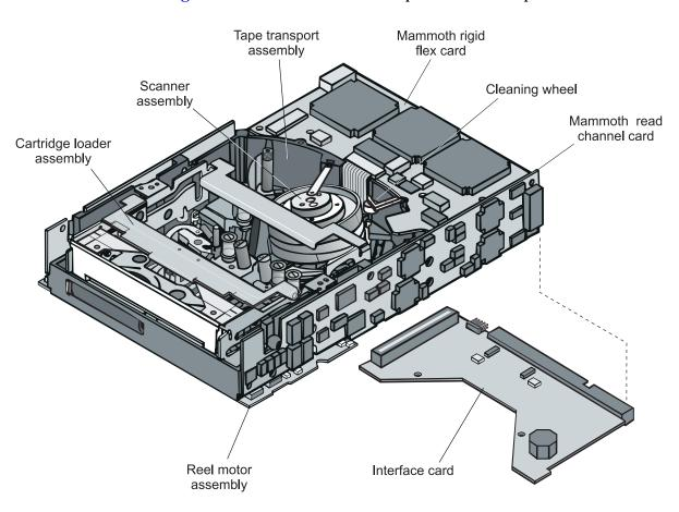
Figure 1-6 shows the internal components of the tape drive.
