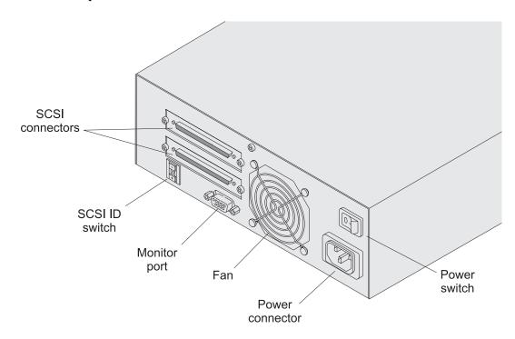
Figure A-4 Back panel components for the tabletop model
