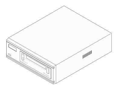
Figure A-1 Tabletop model of the tape drive
