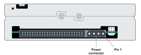
Figure 2-6 Power connector location (single-ended narrow)
