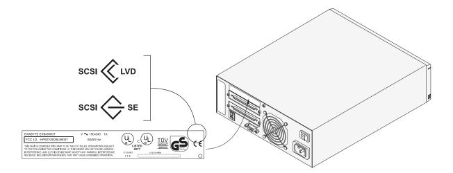
Figure A-6 SCSI configuration on FCC label
