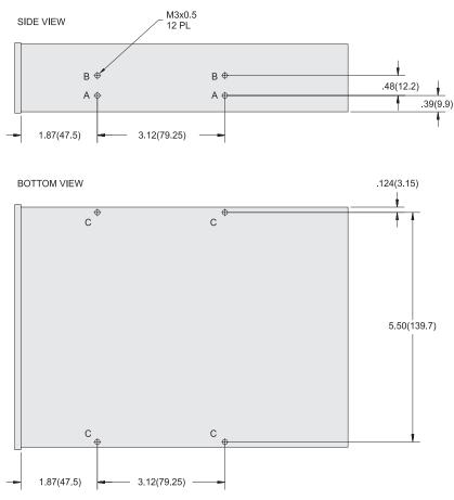
Figure 2-4 Mounting hole dimensions in inches (and millimeters)
