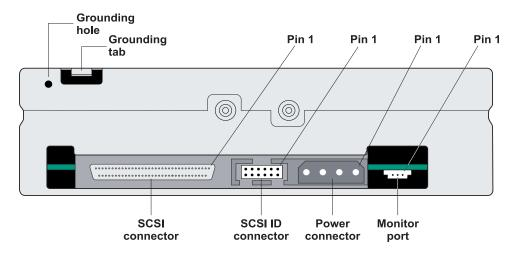
Figure 1-5 Wide SCSI: back-panel components
