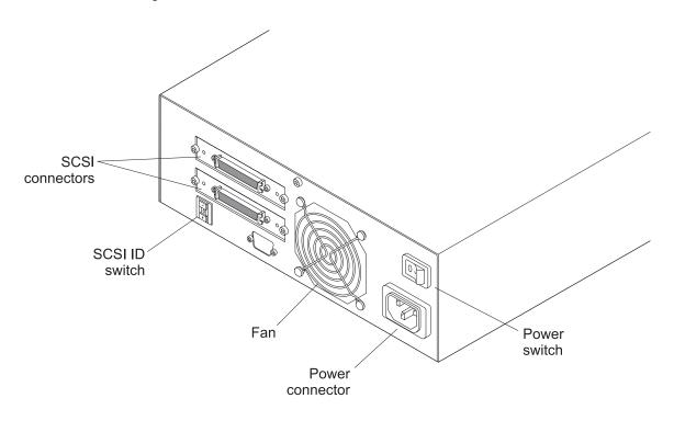
Figure A-3 Back panel of the tabletop tape drive
