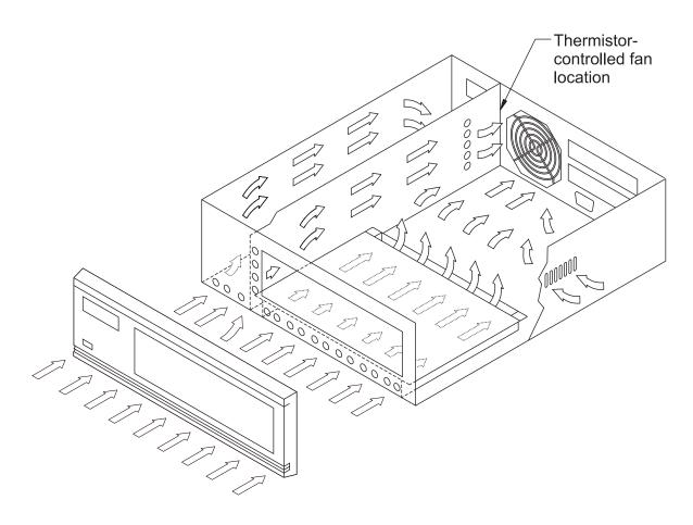
Figure A-7 Air flow through the tabletop enclosure
