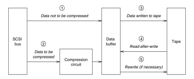
Figure 3-1 Data flow during a write operation
