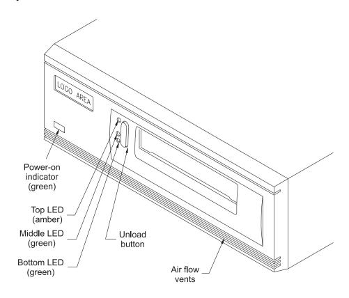
Figure A-2 Front panel of the tabletop tape drive
