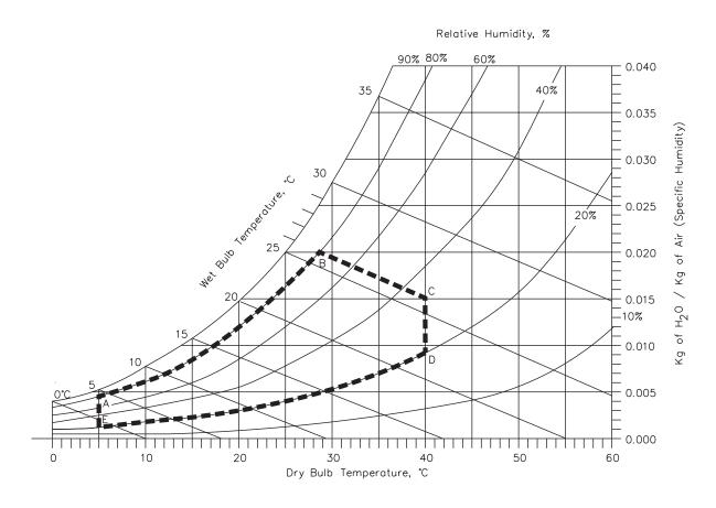
Figure 6-1 Tape path temperature and humidity ranges for operation
