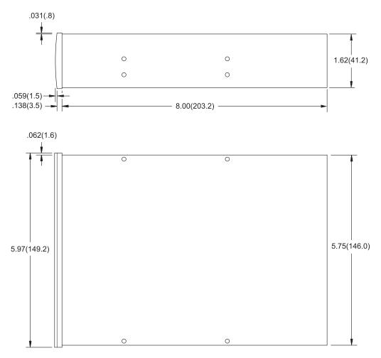
Figure 1-7 Dimensions of the internal tape drive in inches (and mm)
