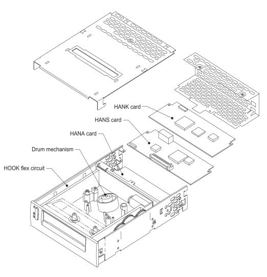
Figure 1-5 Internal components
