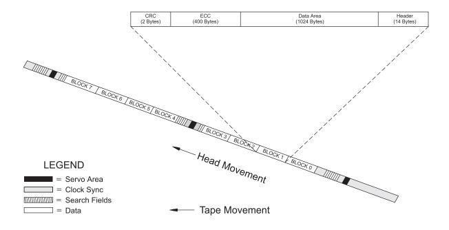
Figure 2-4 Physical block format
