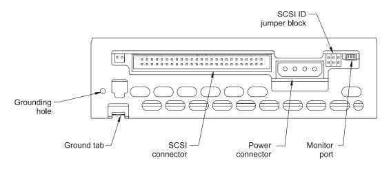
Figure 1-4 Back panel of the internal tape drive
