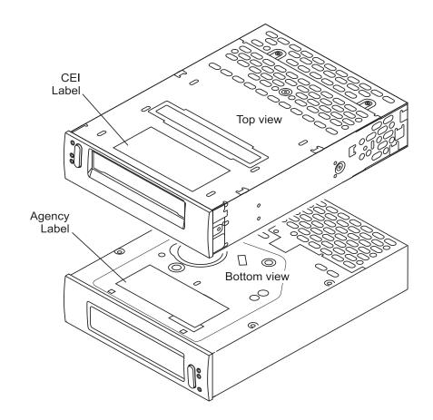
Figure 1-3 Labels on the internal tape drive
