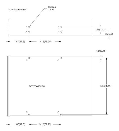
Figure 4-4 shows the dimensions for the internal tape drive's mounting holes.
