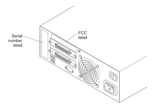
Figure A-4 Labels on the tabletop tape drive
