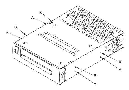
Figure 4-2 Mounting holes on the sides of the internal tape drive
