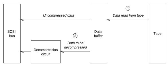
Figure 3-2 Data flow during a read operation
