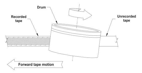
Figure 2-1 Helical-scan recording
