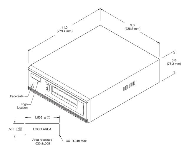
Figure A-5 shows the dimensions of the tabletop tape drive.
