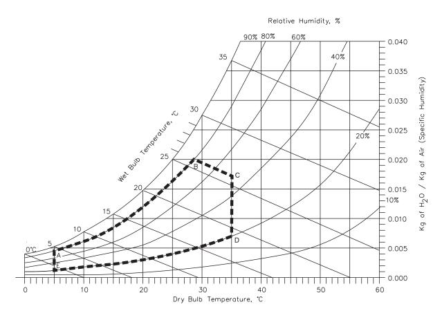
Figure A-6 Ambient operating environment for the tabletop tape drive
