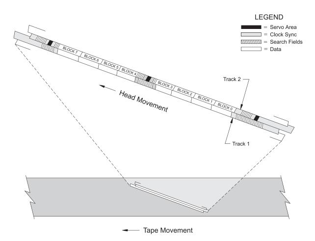
Figure 2-2 8500/8500c physical track structure
