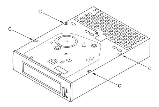
Figure 4-3 Mounting holes on the bottom of the internal tape drive
