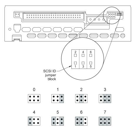
Figure 4-1 SCSI ID jumper block on the back of the internal tape drive
