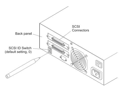
Figure A-8 SCSI ID switch for the tabletop tape drive
