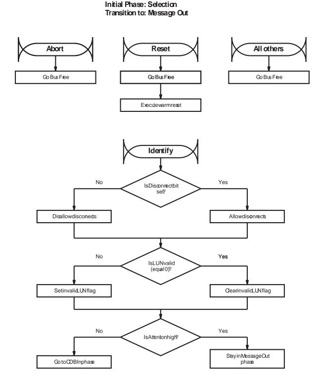
Figure C-1 Message processing after the Selection phase
