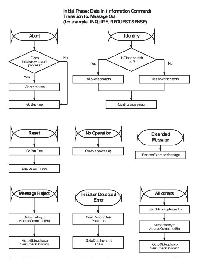
Figure C-10 Message processing during the Data In phase of commands other than READ
