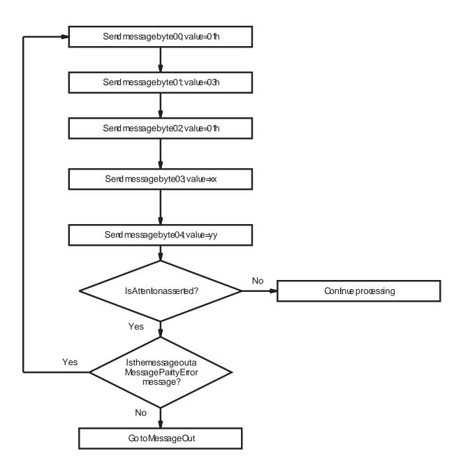
Figure C-6 Message processing for Synchronous Data Transfer Request message
