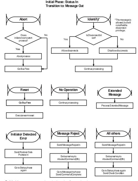
Figure C-11 Message processing during the Status In phase
