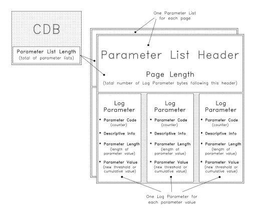
Figure 8-1 Relationship of log parameters and parameter lists to the LOG SELECT CDB
