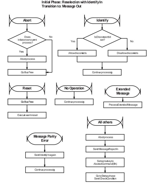
Figure C-13 Message processing after tape drive reselects initiator with Identify message
