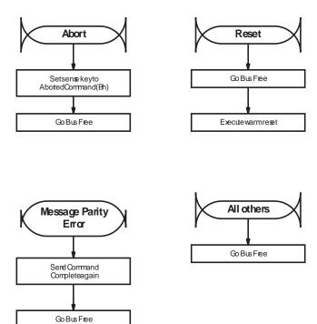
Figure C-12 Message processing during Command Complete Message In phase
