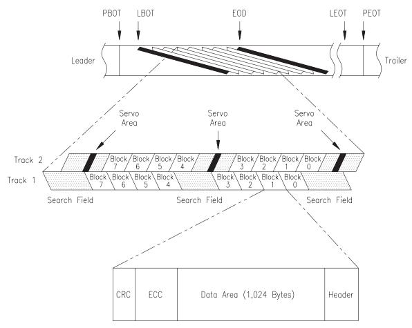
Figure A-2 Structure of data on tape (8500/8500c physical format)
