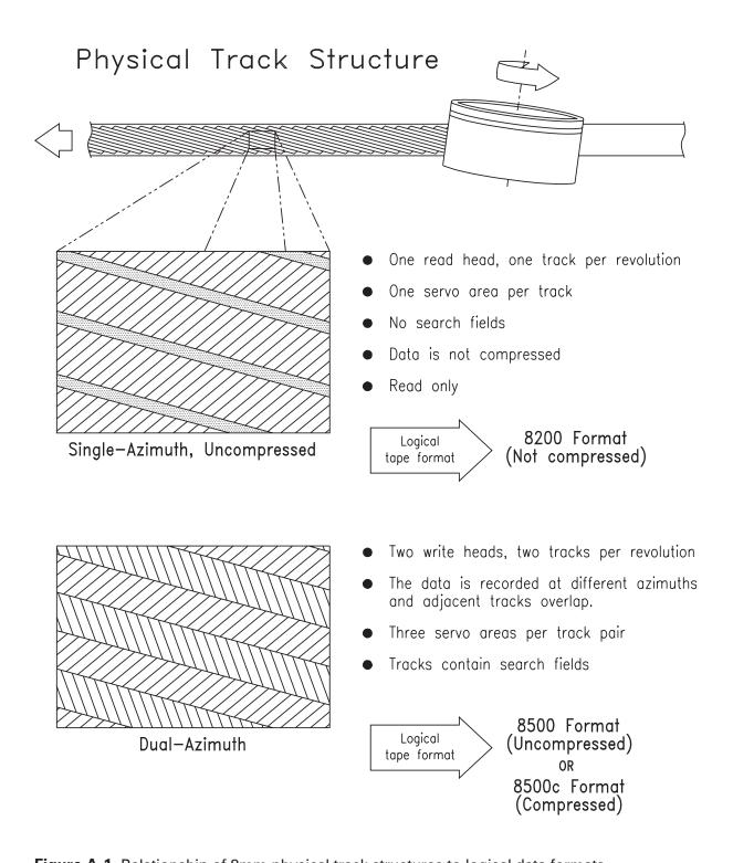
Figure A-1 Relationship of 8mm physical track structures to logical data formats
