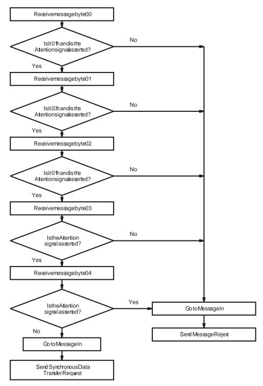
Figure C-5 Message processing of Extended Message Out bytes
