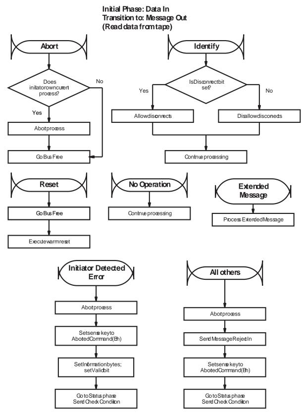
Figure C-9 Message processing during the Data In phase of a READ command
