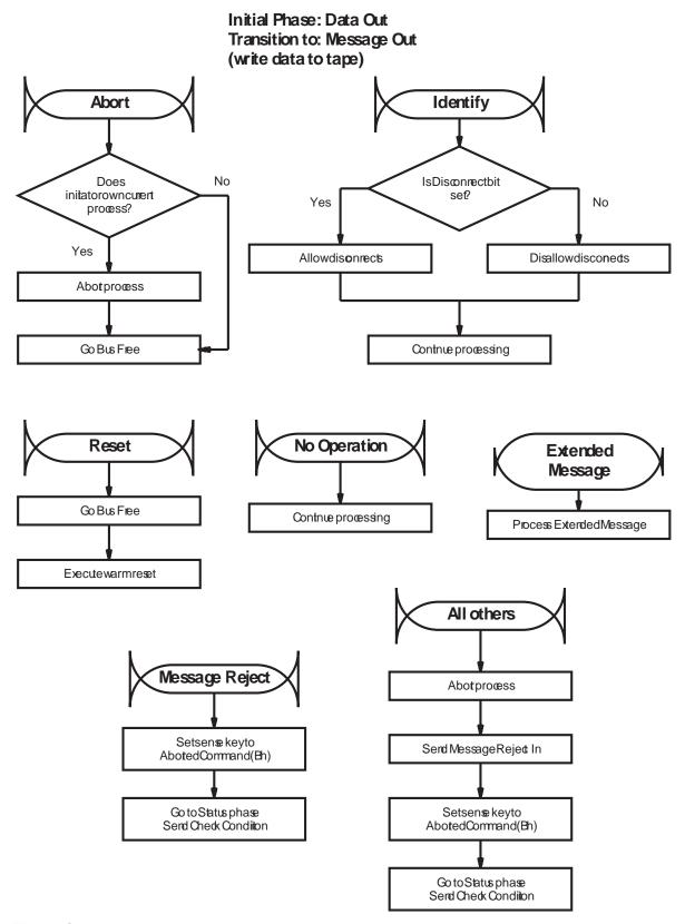
Figure C-7 Message processing during the Data Out phase of a WRITE command
