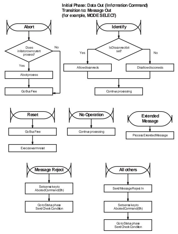
Figure C-8 Message processing during the Data Out phase of a MODE SELECT command
