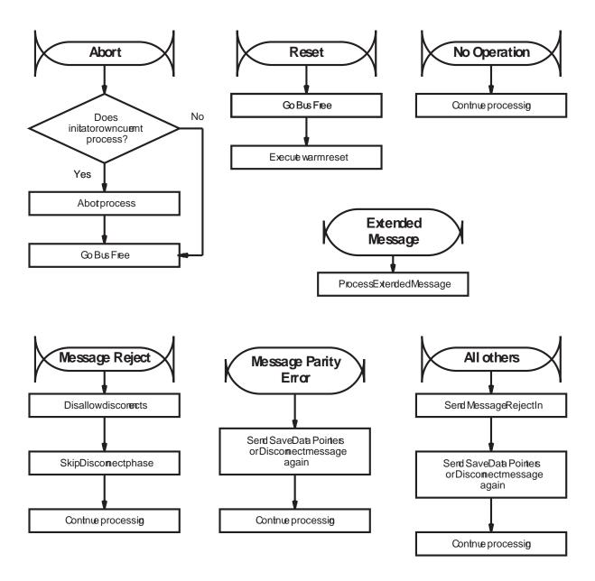
Figure C-14 Message processing while tape drive is executing the Disconnect sequence
