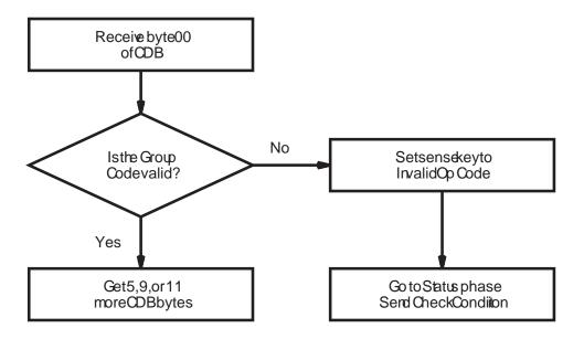
Figure C-3 Processing of CDB bytes
