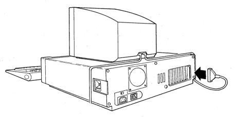
Figure 15: Connecting the Shielded Round Cable to the Tape Controller Card
