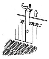
Figure 4: Removing a Slot Cover
