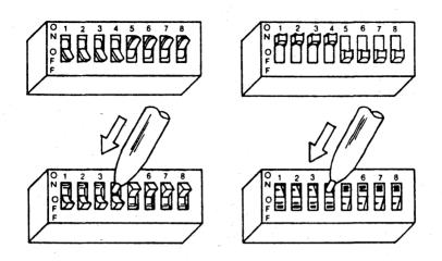
Figure 25: Setting Slide and Rocker Switches
