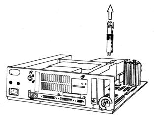
Figure 19: Removing a Slot Cover from the Model 50
