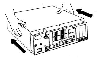
Figure 18: Removing the Cover of the Model 50
