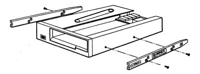
Figure 10: Attaching AT Slide Rails to an Internal Tape Drive
