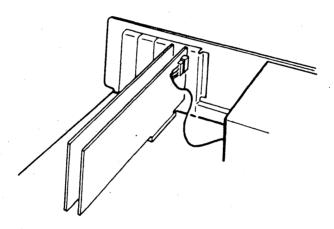
Figure 16: Applying Power to the Tape Controller
