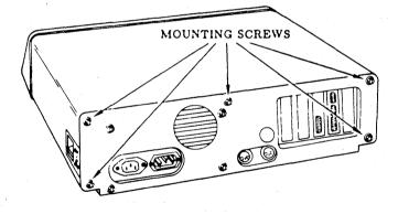
Figure 2: Cover Mounting Screws
