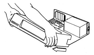
Figure 12: Removing the Cover
