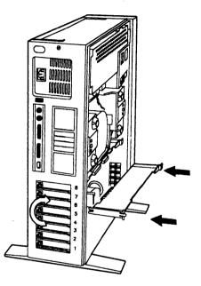
Figure 23: Installing the Tape Controller Card in the Model 60
