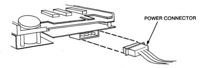
Figure 8: Applying Power to the Tape Drive
