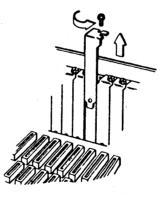
Figure 13: Removing a Slot Cover
