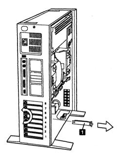
Figure 22: Removing a Slot Cover from the Model 60
