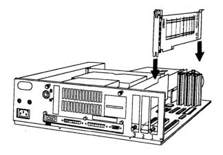
Figure 20: Installing the Tape Controller Card in the Model 50
