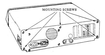
Figure 11: Cover Mounting Screws
