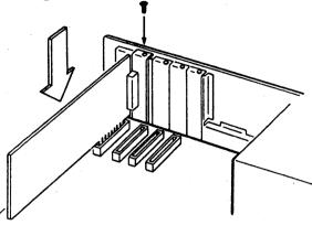
Figure 14: Installing the Tape Controller Card
