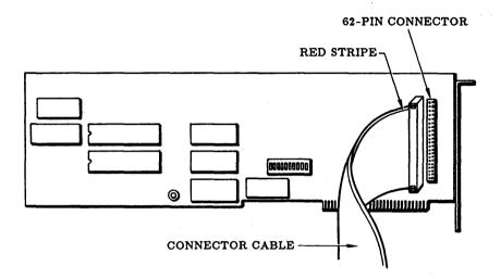
Figure 5: Connecting the Ribbon Cable
