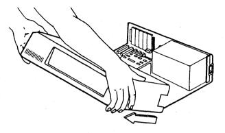
Figure 3: Removing the Cover
