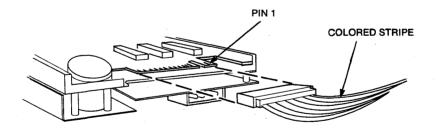
Figure 7: Connecting the Ribbon Cable to the Tape Drive
