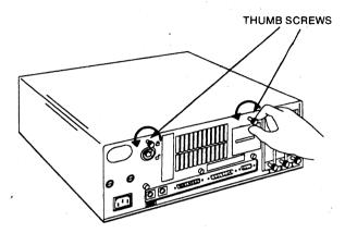
Figure 17: Model 50 Cover Mounting Thumb Screws
