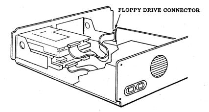
Figure 26: Connecting the Floppy Controller Cable to the Combination Tape/Floppy Controller Card
