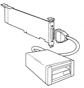
Figure 24: Cabling the Tape Drive and Controller Card
