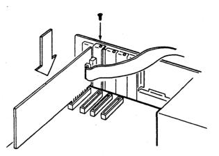
Figure 6: Installing the Tape Controller Card
