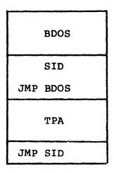
Figure 1-2. Memory Configuration After SID Loads
