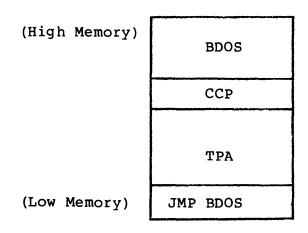
Figure 1-1. Memory Configuration Before SID Loads
