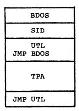
Figure 1-4. Memory Configuration Following Utility Load
