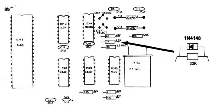
NOTE: These modifications are necessary only on Revision "C" or earlier CPU boards.
