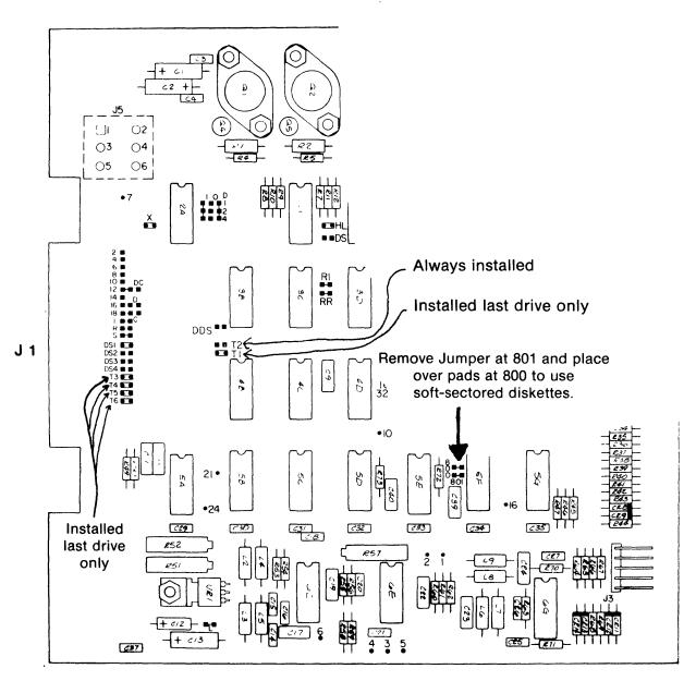
Jumper Plug Installed as Shipped
