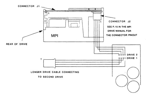
Install the 34-conductor cable in the cabinet matching pin 1 of each cable plug end to the pin 1 end of connector J1 on each drive. Connect the paddlecard end of the cable to the CPU backplane slot designated for the mini-floppy. The backplane of the CPU is wired identically for mini-floppies as for standard floppy drives with the exception of the MOTOR ON line, pin 10. Remove Molex pin from pin 18 and move it to pin 19 of 36-pin edge connector.
