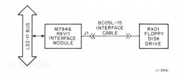
Figure 1-1 RXV11 Floppy Disk System Components
