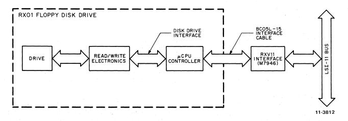
Figure 4-1 RXV11 System Block Diagram
