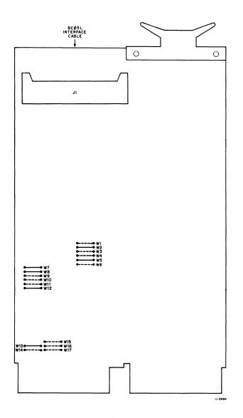
Figure 2-7 RXV11 Device Register and Interrupt Vector Jumper Locations
