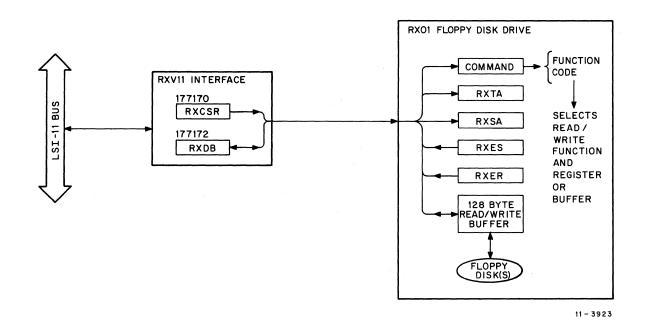
Figure 3-1 RXV11 System Register Functions
