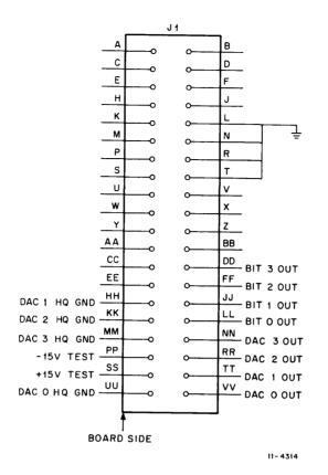
Figure 4-3 40-Pin Connector Pin Assignments
