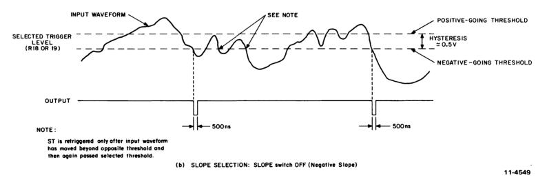
Figure 3-8 KWV11-A Slope Selection
