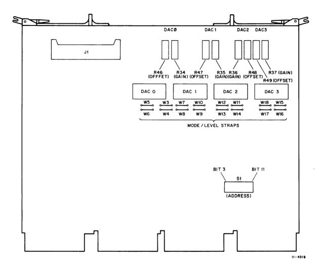
Figure 4-2 AAV11-A Connectors, Switches, and Controls
