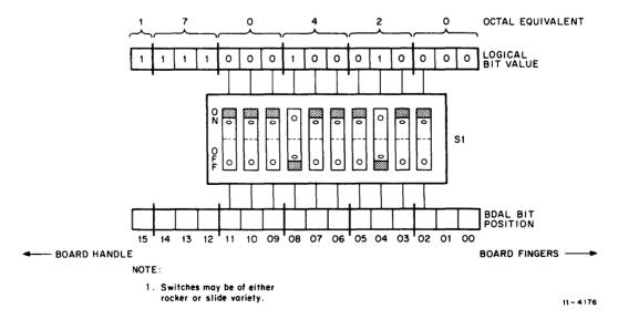
Figure 3-5 KWV11-A CSR Address Switches (Set for 170420)
