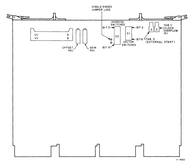
Figure 2-6 ADV11-A Connectors and Switches
