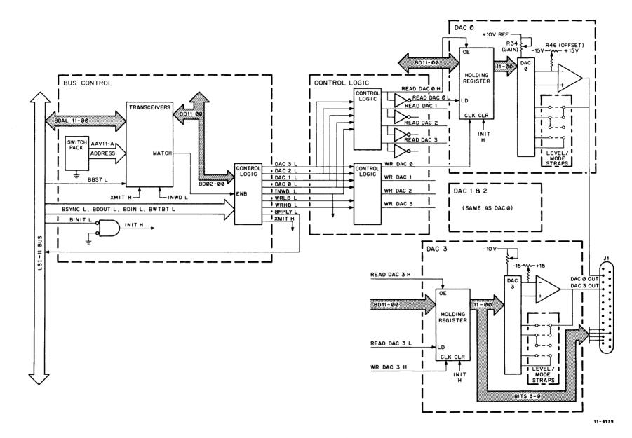
Figure 4-1 AAV11-A Block Diagram
