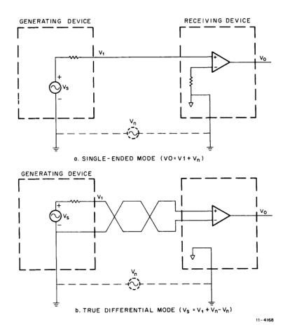
Figure 2-4 Single-Ended Versus True Differential Input Modes
