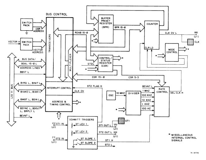
Figure 3-2 KWV11-A Real-Time Clock Block Diagram
