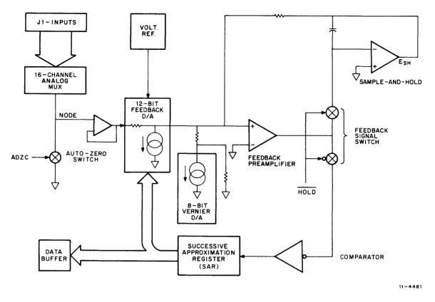
Figure 6-5 ADV11-A A/D Conversion Circuit Block Diagram
