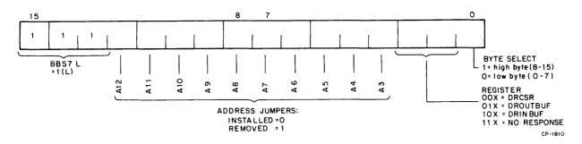
Figure 5-3 DRV11 Device Address
