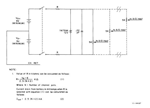
Figure 6-1 Battery-Operated Potentiometer Box for ADV11-A A/D Converter
