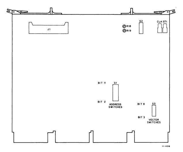
Figure 3-1 KWV11-A Connectors, Switches, and Controls
