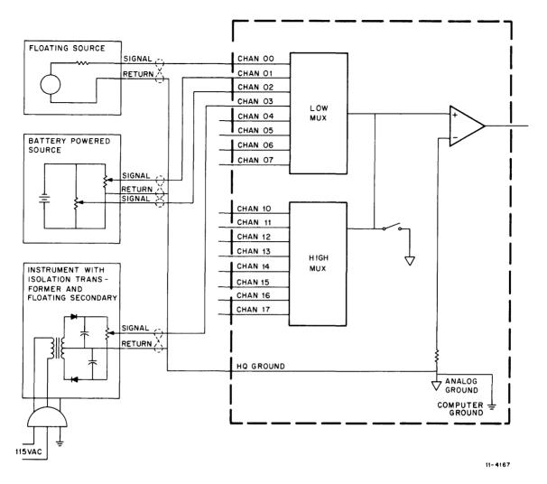
Figure 2-3 Floating ADV11-A Input Signals
