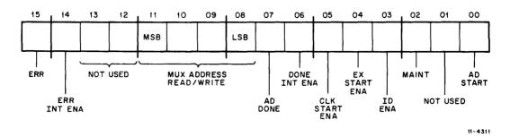
Figure 2-11 ADV11-A Control/Status Register (CSR)
