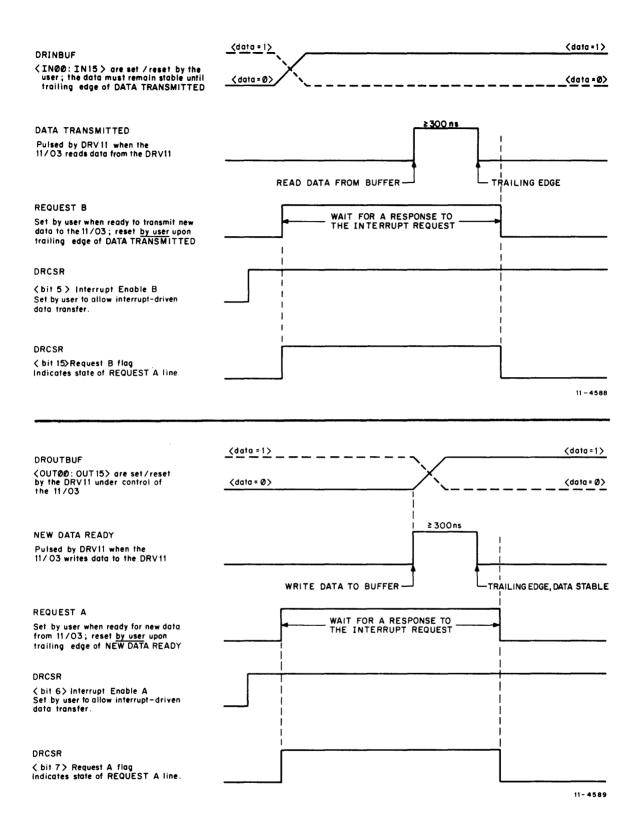
Figure 5-7 DRV11 Interface Signal Sequence
