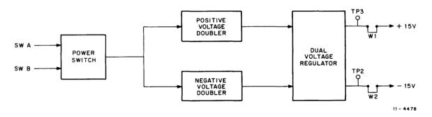
Figure 6-2 Analog Power Supply Block Diagram
