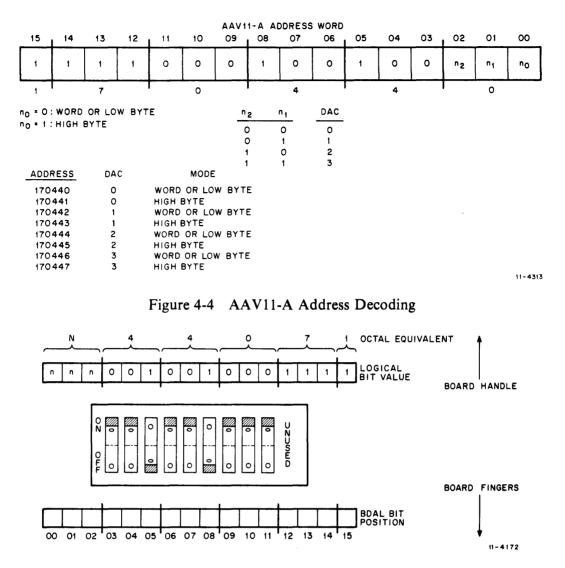
Figure 4-5 AAV11-A Address Switches (set for 17044n)
