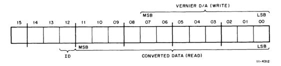
Figure 2-12 ADV11-A Data Buffer Register (DBR)
