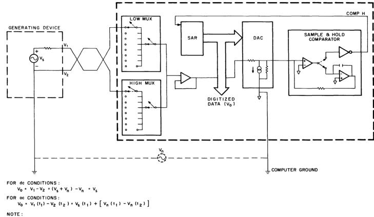
Solid switch positions indicate sample state  $(t_1)$ ; dotted positions indicate hold state  $(t_2)$
