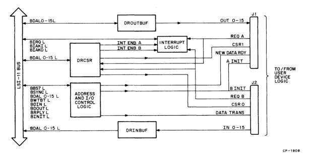
Figure 5-1 DRV11 Parallel Line Unit
