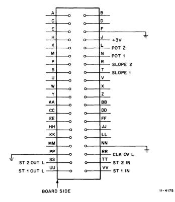
Figure 3-4 40-Pin Connector Pin Assignments
