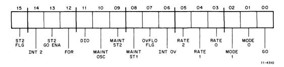
Figure 3-9 CSR Bit Assignments
