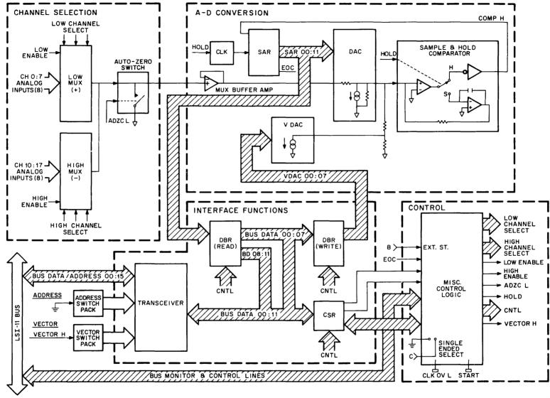
Figure 2-1 ADV11-A Functional Block Diagram
