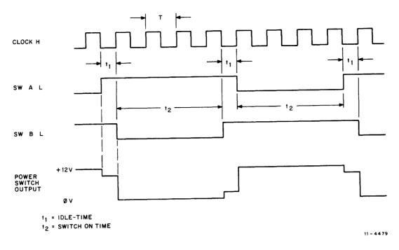
Figure 6-3 DC-DC Converter Signals
