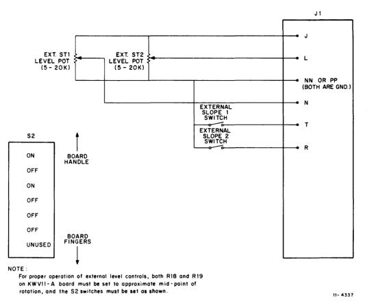
Figure 3-3 Connecting External User-Supplied Slope and Level Controls
