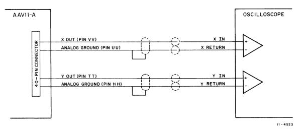
Figure 4-6 Connection to Oscilloscope with Differential Input
