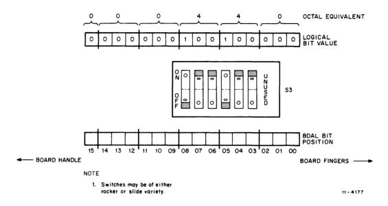
Figure 3-6 KWV11-A Vector Address Switches (Set for 000440)
