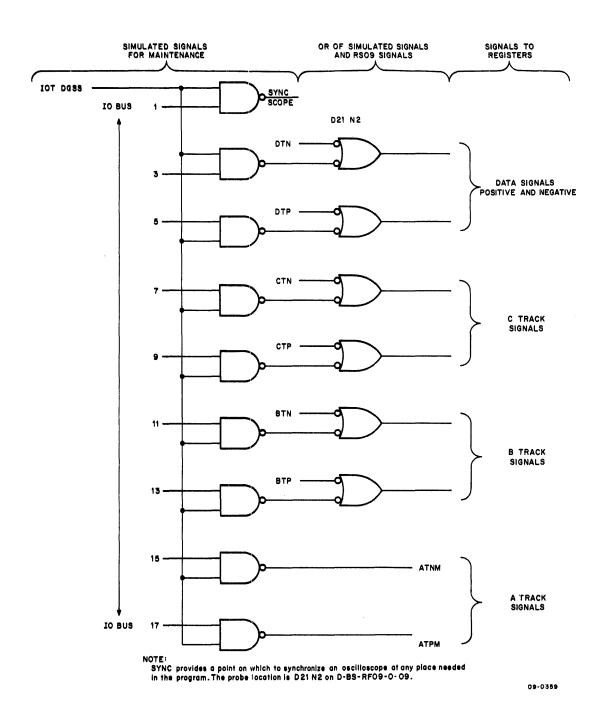
Figure 2-6 Simulating the RS09 with the Maintenance Logic
