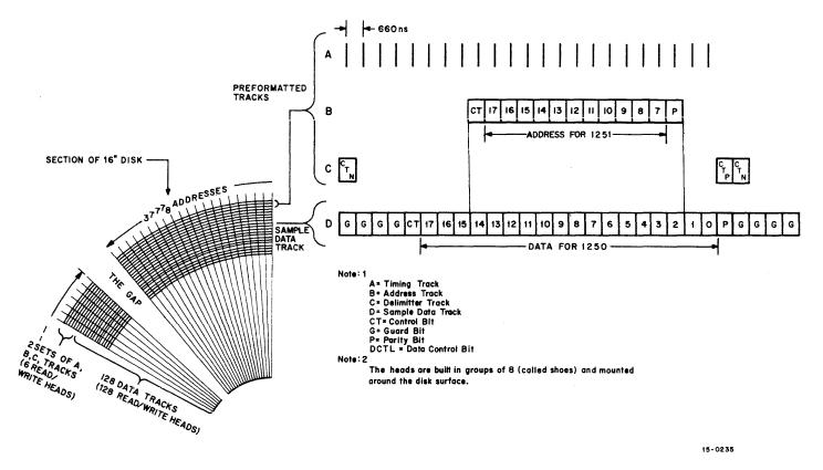
Figure 2-2 Disk Surface Recording Format
