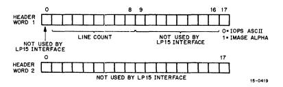
Figure 5-1 Data Buffer Header Format
