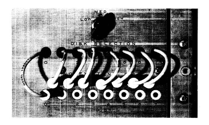
Figure 2–9 Transfer Rate Selection Switch and Disk Address Select Jacks
