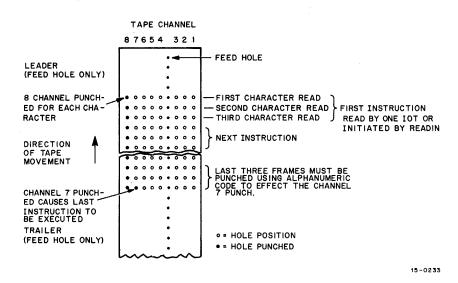
Figure 1-2 HRI Tape Format and Accumulator Bits (Binary Mode)
