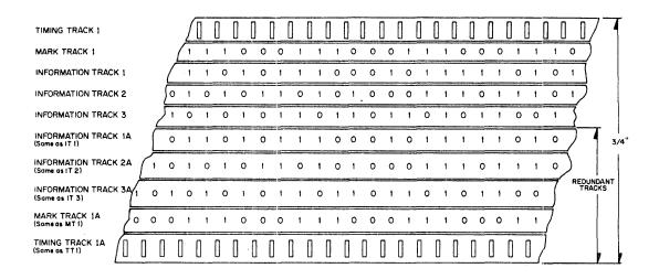
Track Allocation Showing Redundantly Paired Tracks
