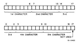
Figure 5-2 5/7 ASCII Packing Scheme
