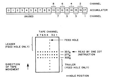
Figure 1-1 Tape Format and Accumulator Bits (Alphanumeric Mode)
