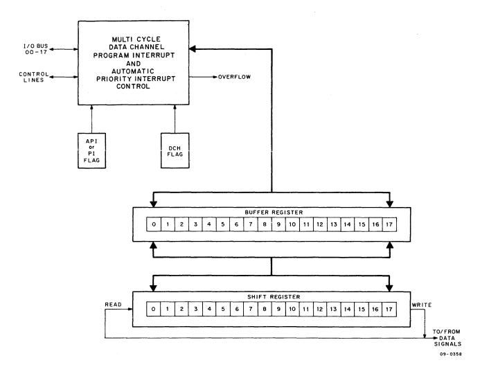
Figure 2-4 DECdisk Data Transfer Section
