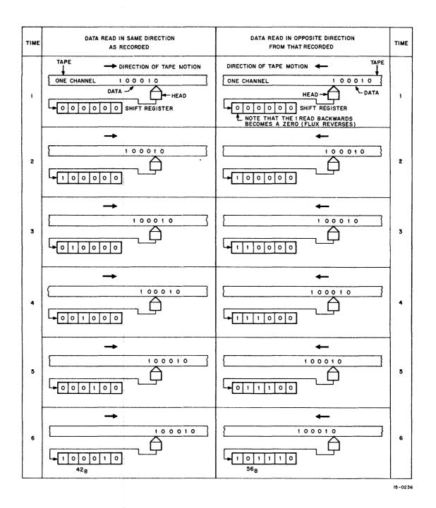
Figure 3-3 Bidirectional Reading and Writing
