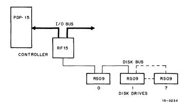
Figure 2-1 DECdisk System Configuration
