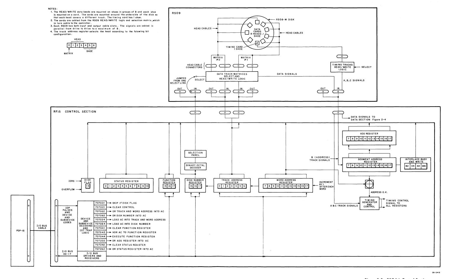
Figure 2-3 DECdisk Control Section
