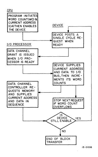
Figure 5–4 Single-Cycle Block Transfer Flowchart
