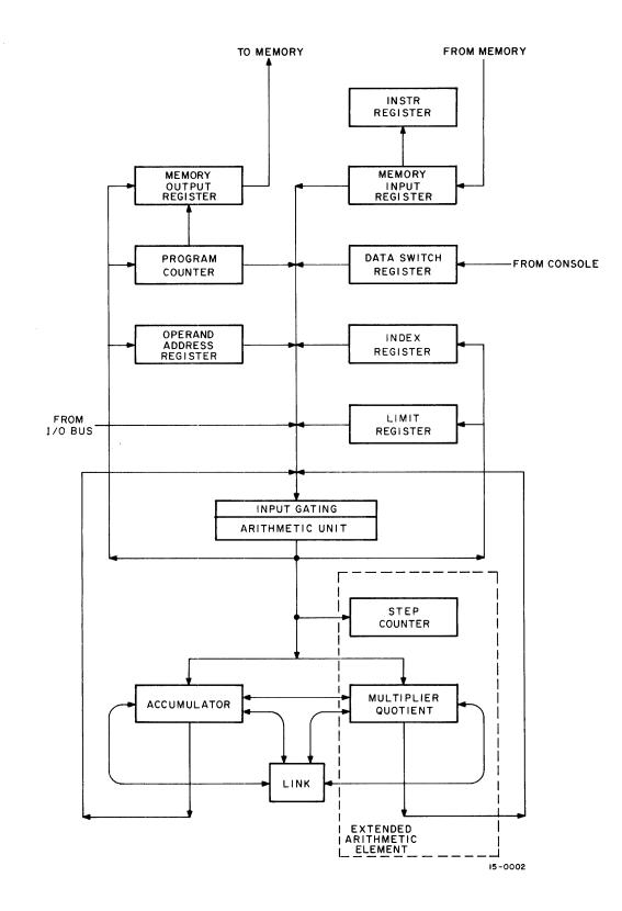
Figure 2-1 Central Processor, Simplified Block Diagram
