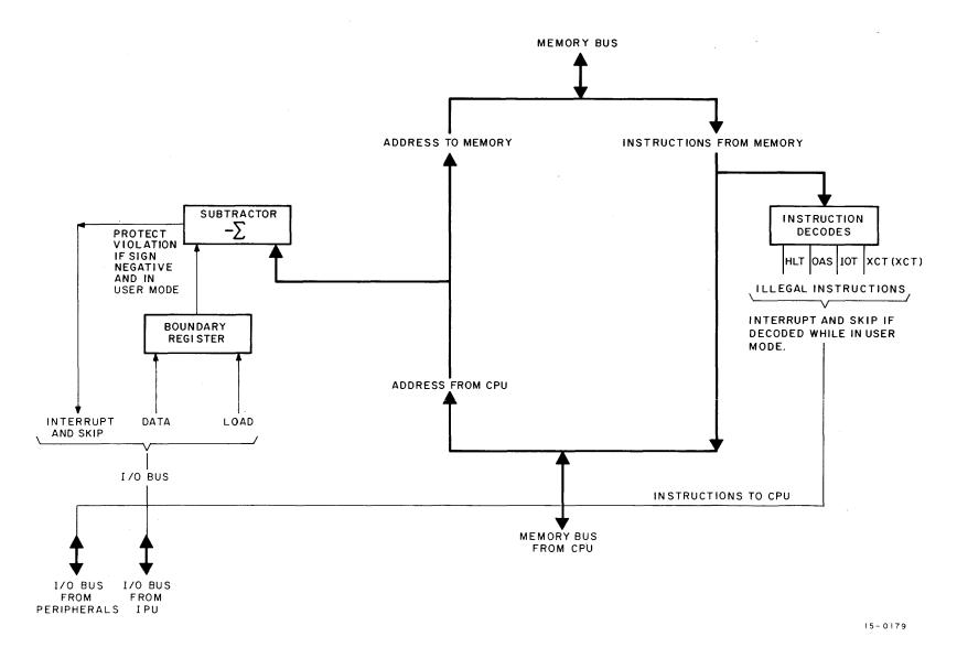
Figure 2–3 Memory Protect Block Diagram
