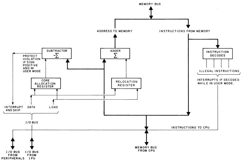
Figure 2-4 Memory Protect and Relocate Block Diagram
