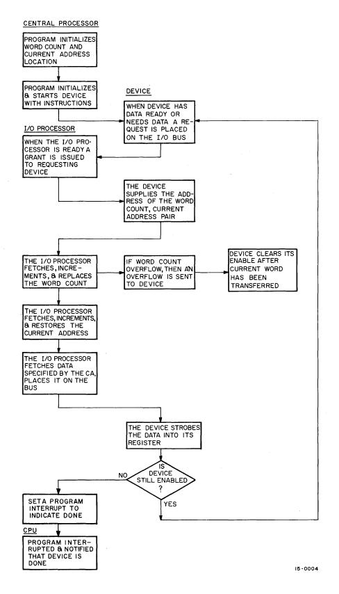
Figure 5-1 Multicycle Out Block Transfer, Flowchart
