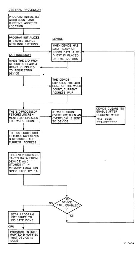
Figure 5-2 Multicycle In Block Transfer, Flowchart
