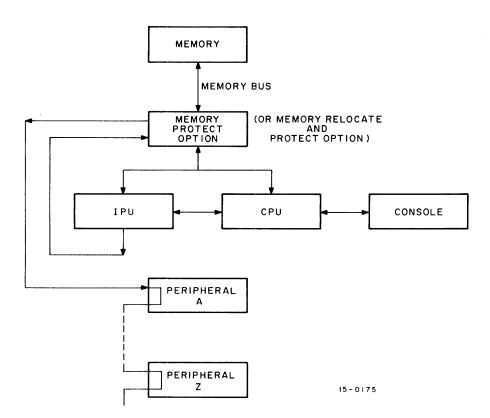
Figure 2-2 PDP-15 System With Memory Protect Option
