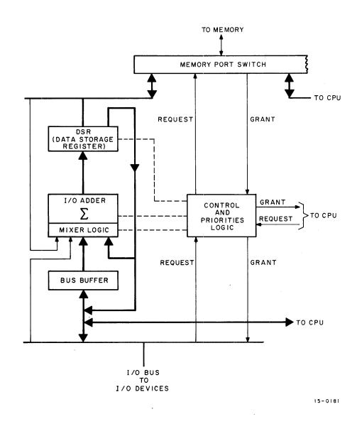
Figure 2–6 I/O Processor Block Diagram
