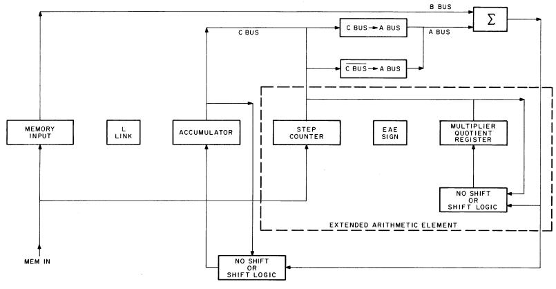
Figure 6-6 EAE Simplified Block Diagram
