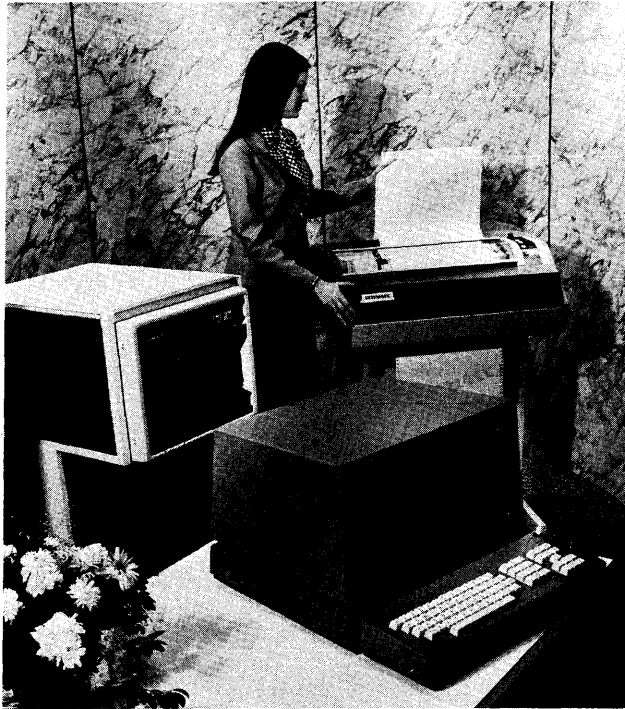
This Ultimacc Disc System features a Data General 1200 minicomputer, a Centronics line printer, and 5 million bytes of disc storage (expandable to as much as 126 million bytes). Ultimacc supplies the hardware interfaces, standard software, and custom programming, and sells the system on a turnkey basis for accounting applications in small businesses.
