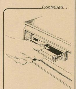
Figure 3-6: Grasping the tape cartridge
