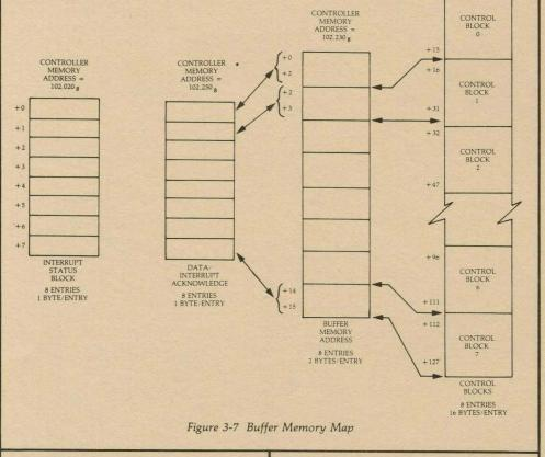
Controller operations are started by writing a control block into the controller memory. The control block contains the following information:
