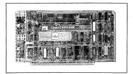
16 BIT 68000 WITH PROVISIONS FOR MMU AND UP TO 16K BYTES OF ROM CLOCK RATES TO 10 MHz CPU 68K TECHNICAL MANUAL Copyright 1982 CompuPro Hayward, CA 94545
