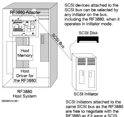
Figure 18 RF3880 in Target Mode
