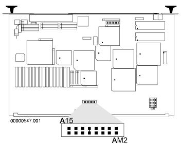
Figure 9 VMEbus Address Jumper
