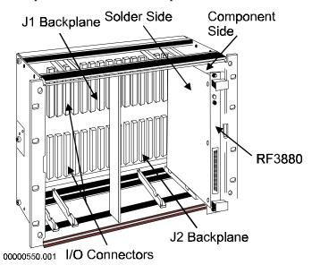
Figure 12 Inserting the RF3880
