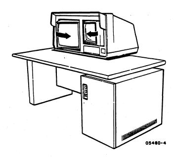
7) At the top of the display cover is an anti-glare hood, which when extended, will minimize glare on the display screens from overhead lights. When overhead lights are not a problem, the hood may be pushed in toward the display cover.
