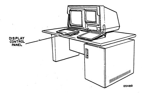
10) The BRIGHTNESS and CONTRAST controls adjust the intensity of the image on the text display. The BRIGHTNESS COLOR control adjusts the brightness of the color display. You will use these controls to adjust the brightness of the displays so messages and images are easily seen but are not excessively bright.
