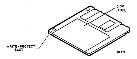
14) With the disk label up, insert the metal edge of the disk into the drive and push the disk into the drive until the disk seats. If there wasn't a disk in the drive, find the diagnostic disk, be sure the write-protect slot is open, and insert the disk (label up, metal edge first) into the disk drive. (With the write-protect slot open, you cannot accidentaly write over and destroy the microcode on the disk.)
