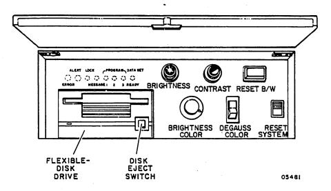
12) When you look at a flexible disk, what you actually see is the case covering the flexible disk. Inside the case, there really is a disk of material upon which information (text, numbers, programs, etc.) can be magnetically recorded. The disk drive rotates the disk within the case and also writes information on or reads information from the disk.
