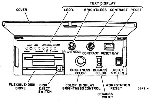
11) Is there a flexible disk already in the flexible-disk drive? (Flexible disks are sometimes called "floppys," or "diskettes," or sometimes just "disks.") If you can't tell by looking or if you can see there is a flexible disk in the drive, press the Disk Eject switch. If a disk is in the drive, the disk will pop part way out so you can remove it.
