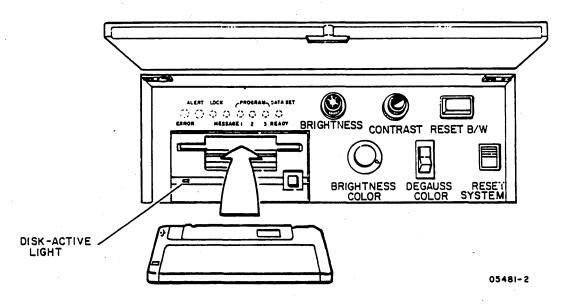
If you leave the display control panel cover up after inserting the disk, you will see the red disk-active light come on momentarily to indicate the workstation is ready to read the disk.
