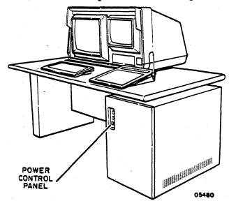
2) If the PROCESSOR ON switch is lit, the workstation is turned on. If the PROCESSOR ON switch is not lit, press the PROCESSOR ON switch to turn on the workstation. (If the green PROCESSOR ON light does not light, the circuit breakers may be turned off - see appendix C.)
