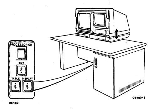
4) Use the DISPLAY switch on the power control panel to raise or lower the displays to the best viewing position. Note that an interlock switch prevents the bottom of the display enclosure from being lowered below the table top.
