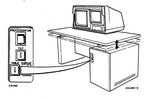
5) Use the TILT switch on the power control panel to tilt the displays backward or forward to the best viewing position.
