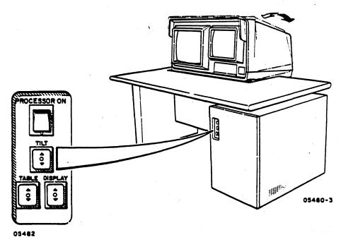
6) The displays also swivel horizontally. Press on the edges of the displays to swivel them to the best viewing angle.
