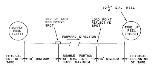
Figure 3. Physical Layout of Tape
