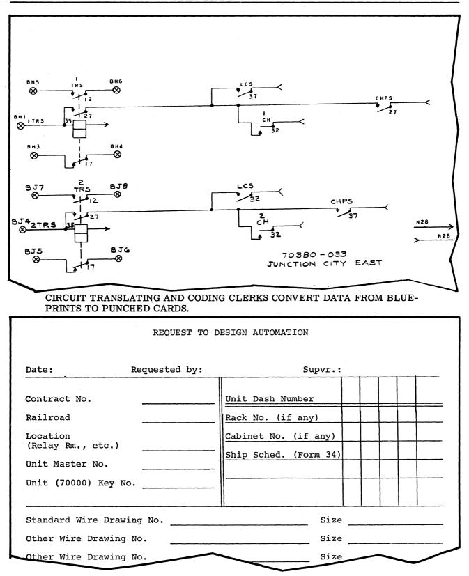
A REQUEST FOR OUTPUT ACCOMPANIES THE BLUEPRINT. DATA FROM THIS FORM ALSO IS KEYPUNCHED AND, IN EFFECT, TRIGGERS THE PROGRAMS REQUIRED TO PRODUCE THE DESIRED OUTPUT.
