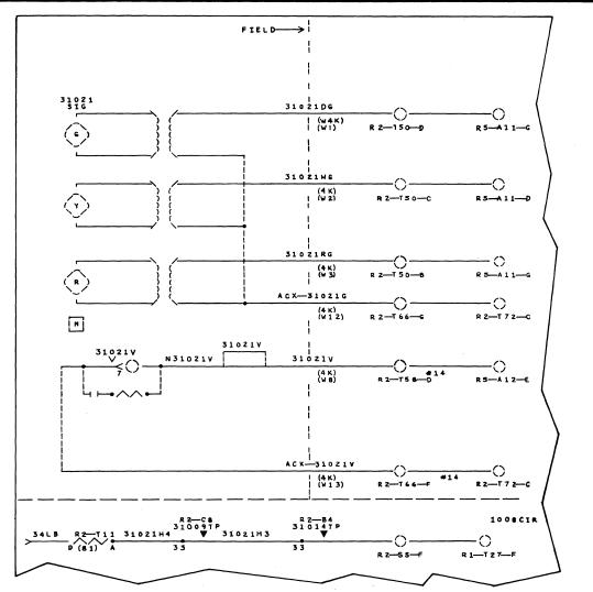
SPECIAL CHARACTER SETS ON THE IBM 1403 PRINTER ENABLE GRS TO PRODUCE SCHEMATICS USED TO ASSEMBLE THE CIRCUITRY IN THE SWITCHES AND CONTROL SYSTEMS IT MAKES. PRODUCTION OF THESE CHARTS BY MANUAL METHODS REQUIRED NEARLY SIX HOURS.
