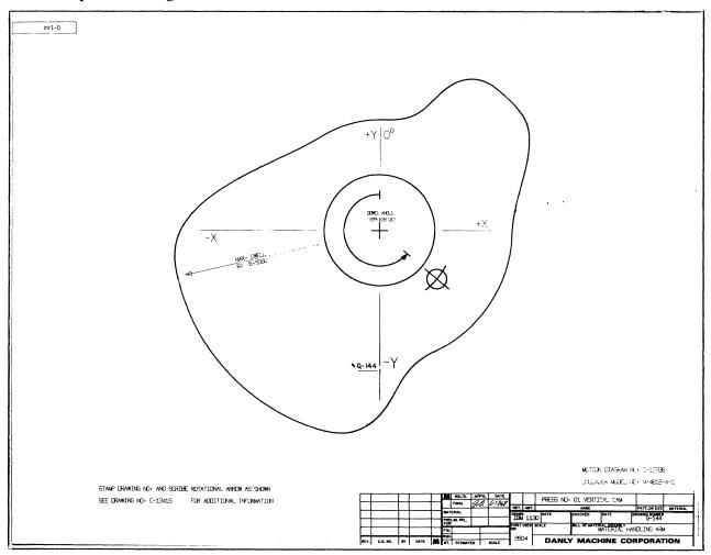
THE DIGITAL PLOTTER, USING THE MOTION DIAGRAM PARAMETERS, GENERATES A PUNCHED PAPER TAPE AND A DRAWING OF THE REQUIRED CAM.
