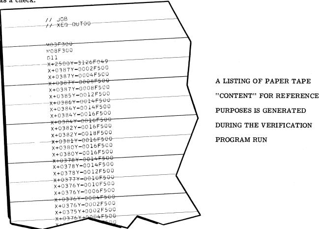
Benefits of machine-generated numerical control tape are speed and accuracy. Hand-punching a tape is a "typographical process open to typographical errors and may take one man-day to complete," explains Carl Tack, director of technical services. In contrast, cards fed into the 1130 generate the same complete numerical control tape in less than five minutes total time, and using fewer rounded-off numbers.
