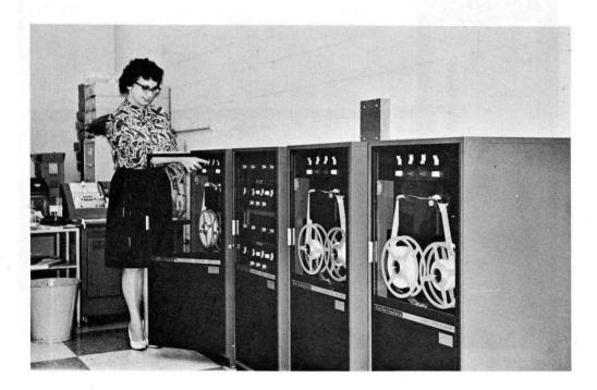
OPERATOR PREPARES TO LOAD A REEL OF PAPER TAPE IN THE RE-CEIVER CONSOLE. ADJOINING UNIT IS THE CENTRAL CONSOLE. Provision is also made in the system for reporting multiple machine operations where a worker operates two or more machines simultaneously and group operations where two or more employes work on the same operation. In addition, reports are made on incompleted operations.
