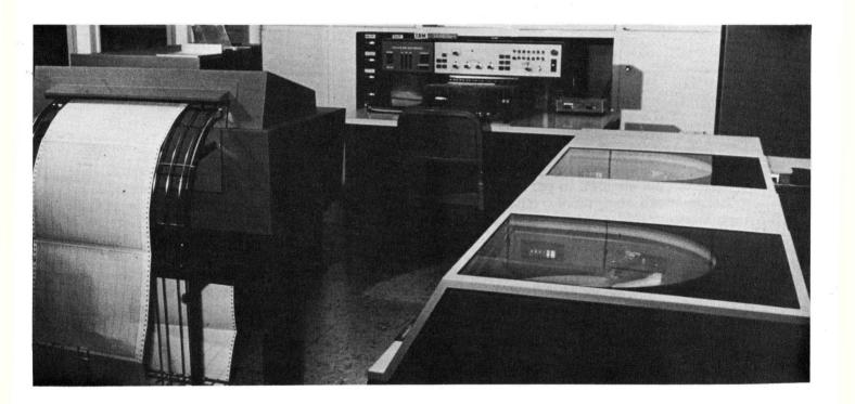
Fig. 1. IBM 1440 DATA PROCESSING SYSTEM used by Sigman includes IBM 1443 card read-punch (upper left), IBM 1443 printer (lower left) and two IBM 1311 disc drives (lower right).
