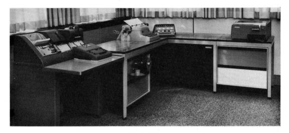
Fig. 1. - MONROBOT XI in its vendor quality rating configuration uses punched card input prepared on IBM 026 keypunch (shown at left). Monro-Card Processor is on top surface right.
