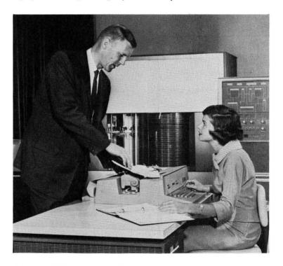
IBM 1405 DISC STORAGE UNIT retains all corporate data and programs in its 25 magnetic discs.
