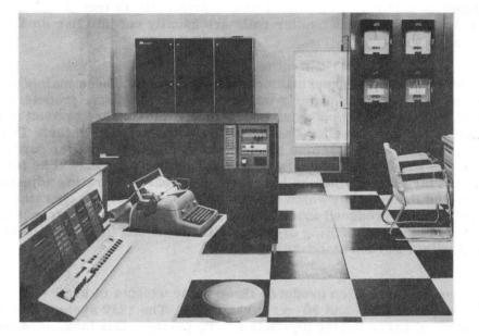
IBM 1710 PROCESS CONTROL SYSTEM which supervises papermaking at Cellulose du Pin's Facture plant, is centered around an IBM 1620 COMPUTER (console at left). Unit at right of window is a French-made analog signal indicator which continuously feeds the computer production line data.
