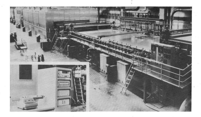
SIXTY ELECTRONIC AND PNEUMATIC COMPUTER INPUT DEVICES are located down the Beloit papermaking machine's 400-foot length. IBM 1717 OUTPUT TYPEWRITERS (see inset) report all 1710 corrective actions to plant floor personnel. Information can be entered manually from plant floor through switch-controlled console, beside typewriter.
