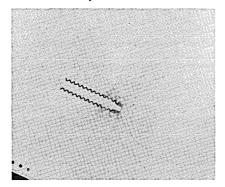
effect upon each grid point, and plotting devices produce "synthetic seismographic patterns" like the one shown in the picture above. When a seismographic pattern thus created resembles one generated by a real earthquake, the research team concludes that the laboratory earthquake was a close approximation of the real quake. They can then draw conclusions about the activity below the earth's surface that triggered the actual jolt.
