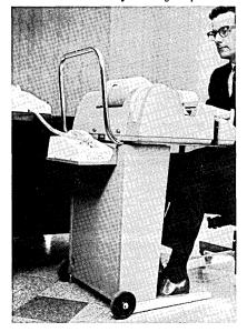
A large range of options include: paper tape input-output; automatic control of paper tape reader and/or punch; friction or sprocket feed; automatic form feed; 74 or 88 columns per line; mobile stand; and separate or built-in acoustic data set providing originate only or originate/answer mode. The portable units are available singly or in quantity lots.
