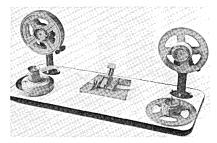
Punch. Tape direction (on a roll) can be changed by transferring from one manual winder to the other or tape direction can be maintained while splicing or editing by using the Center-Feed Unwinder. Datalink Processors are available in many configurations to fit the user's requirements.
