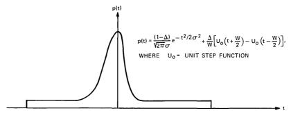
Fig. 15—Gaussian pulse on a pedestal.
