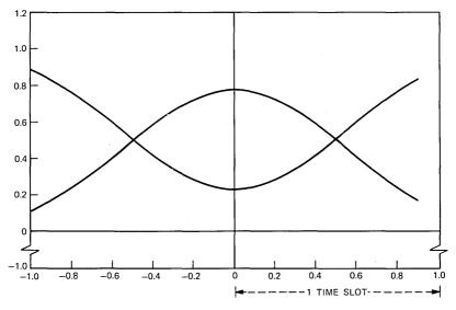
Fig. 5—Eye diagram for gaussian impulse response;  $\sigma/T = 0.35$ .
