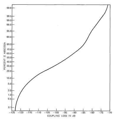
Fig. 4—Distribution of 1000-Hz NEXT coupling loss (dB).
