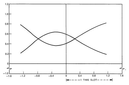
Fig. 12—Eye diagram for borosilicate fiber 740 meters long;  $\sigma/T = 0.60$ .
