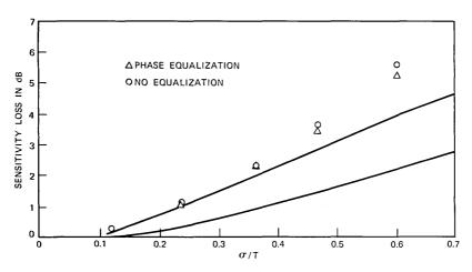
Fig. 13—Sensitivity losses vs  $\sigma/T$  for borosilicate fiber (includes phase equalization).
