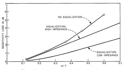
Fig. 10—Sensitivity losses vs  $\sigma/T$  for borosilicate fiber.
