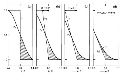
Fig. 4—Power distribution immediately ahead of the splice (q) and immediately behind the splice (p) for various power distributions plotted vs the mode coordinate R. The cross-hatched areas indicate splice loss; D = 0.1.
