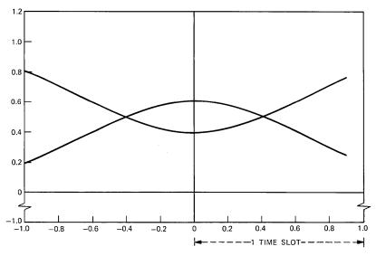
Fig. 7—Eye diagram for gaussian impulse response;  $\sigma/T = 0.55$ .
