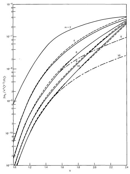
Fig. 3—Normalized loss coefficient of the single-mode, step-index fiber as a function of the normalized frequency parameter V for several values of the power law exponent m. The loss values in this curve correspond to the flat portions on the lefthand side of Figs. 1 and 2. The solid curves correspond to eq. (5) while the dotted curves were computed from the approximate equation (17). The dash-dotted curves represent (17) without the term  $V^m$ .  $n_1 = 1.515$ ,  $n_2 = 1.5$ .
