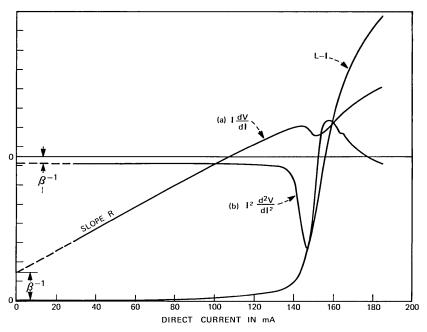
Fig. 2—Typical  $V(\Omega)$  and  $V(2\Omega)$  responses [curves (a) and (b)] as functions of laser current measured using apparatus of Fig. 1. The zero current intercept of I(dV/dI) and the initial negative offset of  $I^2(d^2V/dI^2)$  are proportional to  $\beta^{-1} = (\alpha kT/q)$  when the simple model described in the text is valid. Note voltage saturation in I(dV/dI) and the very strong second-derivative signal near threshold.
