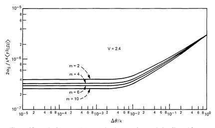
Fig. 1—Normalized loss coefficient of the single-mode, step-index fiber with power spectrum defined by (11) as a function of the width parameter  $\Delta\theta/k$  of the power spectrum. The curve parameter *m* indicates the exponent of the power law.  $n_1 = 1.515$ ,  $n_2 = 1.5$ , V = 2.4.
