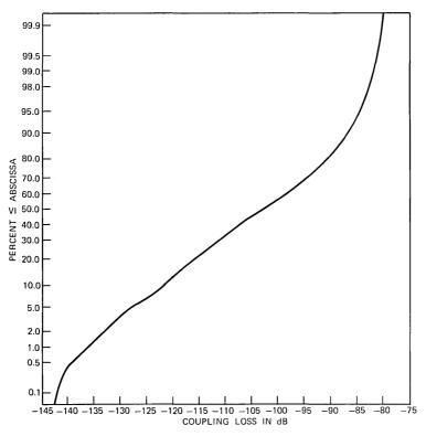
Fig. 10-Distribution of 1000-Hz FEXT coupling loss (dB).
