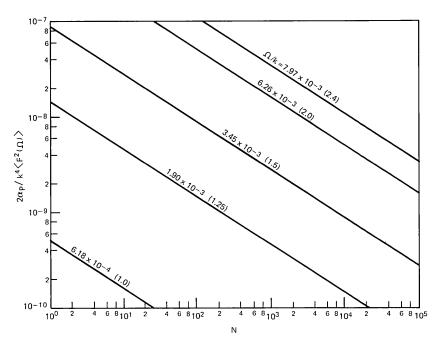
Fig. 5—Normalized loss coefficients of the multimode, parabolic-index fiber which is designed so that its spatial frequency  $\theta_p$  [eq. (24)] coincides with the spatial frequency  $\Omega$  [eq. (3)] of the single-mode fiber. The values of  $\Omega/k$  label the curves; the values shown in parenthesis are the corresponding V values of the single-mode fiber.
