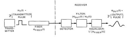
Fig. 1-Equalizing receiver.
