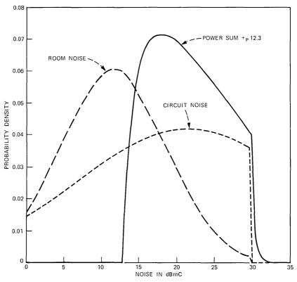
Fig. 5—Power sum of noise sources (gain = 4 dB).
