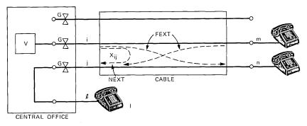
Fig. 2—vFG cable crosstalk coupling path.
