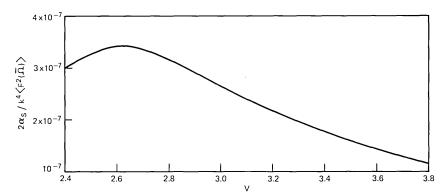
Fig. 4—Plot of eq. (20). This curve represents the normalized radiation loss of a quasi-single, HE<sub>11</sub> mode in the presence of a leaky (next-higher-order) mode. The curve in this figure continues the curves in Fig. 3 to higher values of V,  $n_1 = 1.515$ ,  $n_2 = 1.5$ .
