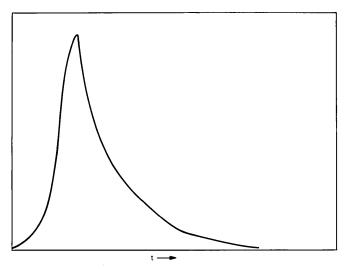
Fig. 9-Impulse response of borosilicate fiber 740 meters long.
