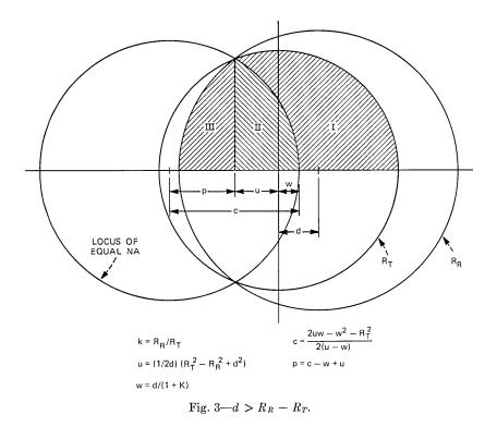
the areas of overlap into sections which are bounded by a circle and a straight line and to combine these sections to obtain the required geometry. All integrals then have the form suggested by eqs. (7) and (8) and can be segmented into the following three integral forms.
