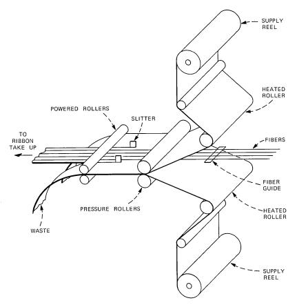
Fig. 2-Laminated fiber ribbon fabrication.
