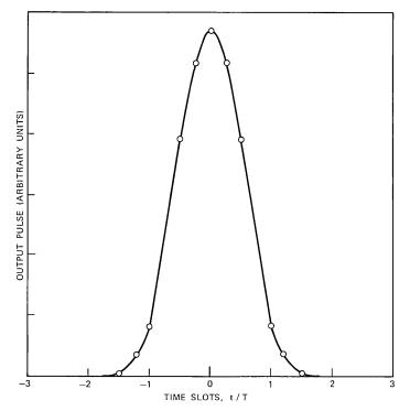
Fig. 6—Receiver output pulse for gaussian impulse response;  $\sigma/T = 0.35$ .
