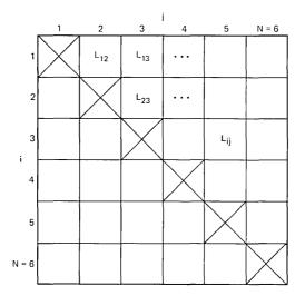
Fig. 3-Symmetric matrix of crosstalk coupling-loss measurements.
