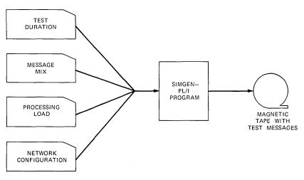
Fig. 4—Process of creating test-message tape.
