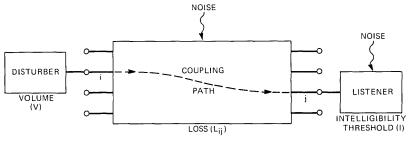
Fig. 1-General crosstalk coupling model.
