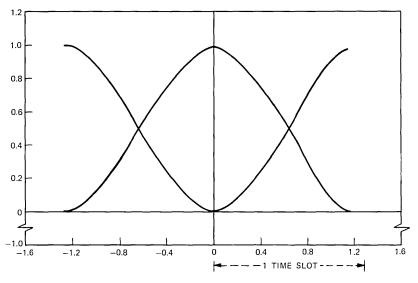
Fig. 2(b)—Ideal eye diagram;  $V_{out}(t)$ , T = 1.28.
