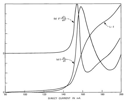
Fig. 3—Typical results for I(dL/dI) and  $I^2(d^2L/dI^2)$  vs current in an (Al, Ga)As double-heterostructure laser taken with the apparatus shown in Fig. 1, except that the signal input to the phase detector was obtained from a silicon detector monitoring the light emission from the laser.
