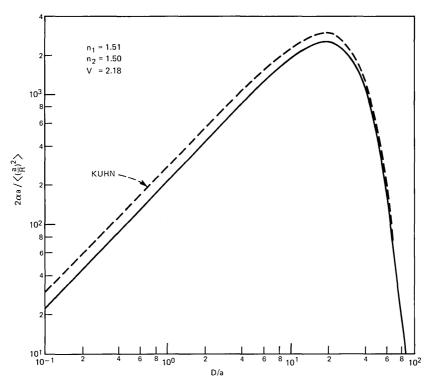
Fig. 10—Comparison between Kuhn's theory and our theory for  $n_1 = 1.51$ ,  $n_2 = 1.5$ , and V = 2.18. The autocorrelation function of the fiber curvature is gaussian.
