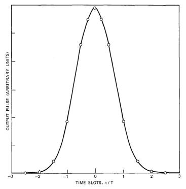
Fig. 8—Receiver output pulse for gaussian impulse response;  $\sigma/T = 0.55$ .
