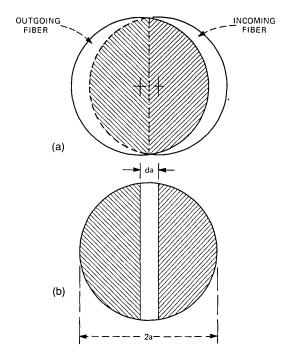
Fig. 1—Areas of transmission in a fiber splice. (a) End-on view of the splice. (b) Area of overlap rearranged for computation of offset loss.
