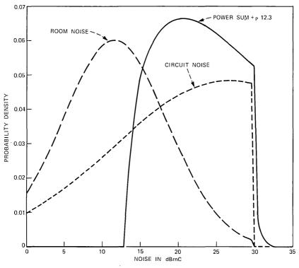
Fig. 7—Power sum of noise sources (gain = 9 dB).
