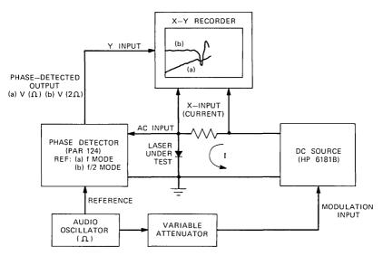
Fig. 1—Schematic diagram of apparatus used to obtain voltage and light derivatives in (Al, Ga)As double-heterostructure lasers. Mode (a) detects  $V(\Omega) \propto I(dV/dI)$ and mode (b) detects  $V(2\Omega) \propto I^2(d^2V/dI^2)$ .
