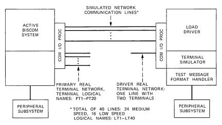
Fig. 3—Example of the active and load-driver configuration.
