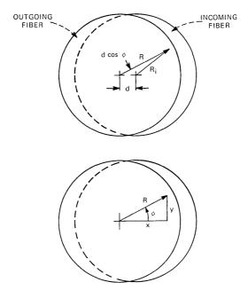
Fig. 3—Coordinate system used to compute offset loss.
