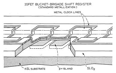
Fig. 3-Cutaway view of integrated bucket-brigade register-standard metallization.
