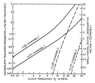
Fig. 12—Theoretical incomplete transfer parameter versus clock frequency for minimum size bucket-brigade shift register.
