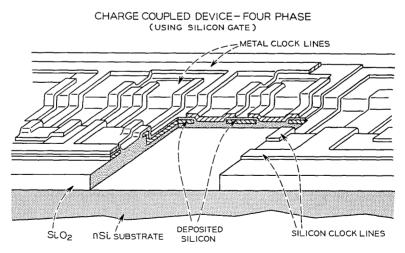
Fig. 8-Sectional drawing of a multilevel charge-coupled device.
