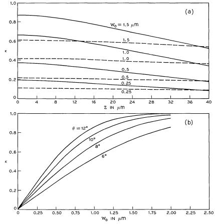
Fig. 11—(a) Power coupling coefficient,  $\kappa$ , is plotted versus axial separation, z, between a laser and a single-mode fiber ( $\lambda = 9000$  Å). The half-width,  $w_o$ , of the laser beam waist is the parameter. Solid curves apply to a 3.2- $\mu$ m fiber (mode radius = 2.6  $\mu$ m). Dashed curves apply to a 3.7- $\mu$ m fiber (mode radius = 4.6  $\mu$ m). (b)  $\kappa$  is plotted versus  $w_o$  ( $\lambda = 9000$  Å). Fiber acceptance angle,  $\theta$ , is the parameter.
