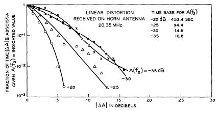
Fig. 13-Conditional linear distortion distributions for 20.35 MHz.
