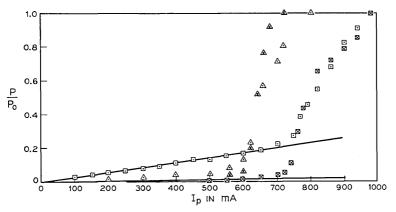
Fig. 6—Normalized power radiated from the laser surface versus pump current:  $\Box$  L-352 #1, DH laser with oxide-masked stripe;  $\triangle$  L-363 #1, DH laser with protonbombarded stripe. Normalized power leaving the end of a 3.2- $\mu$ m fiber versus pump current:  $\boxtimes$  L-352 #1, DH laser;  $\triangle$  L-363 #1, DH laser.
