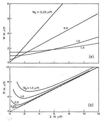
Fig. 10—(a) The half-width, w, of a Gaussian beam is plotted versus z, the separation of the reference plane from the plane of the beam waist ( $\lambda = 9000$  Å). The half-width,  $w_0$ , of the electric field at z = 0 is the parameter. (b) The wavefront radius of curvature, R, is plotted versus z ( $\lambda = 9000$  Å).  $w_0$  is the parameter.
