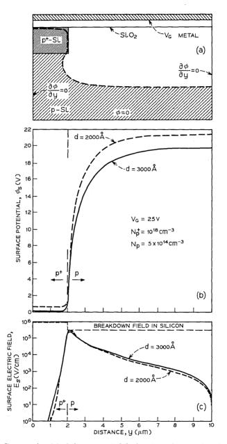
Fig. 7—Cross section (a) of charge-coupled device electrode normal to the channel direction showing channel-stop diffusion as used in computer analysis. Surface potential (b) and surface electric field (c) across channel-stop boundary for fixed electrode voltage and two oxide thicknesses.
