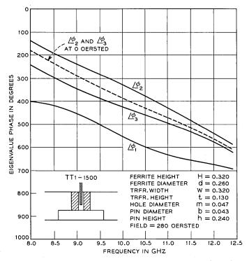
Fig. 22—The eigenvalue phase-frequency response of a junction with a transformer and pinned, full height ferrite. The eigenvalues have been linearized by the transformer in the vicinity of the  $TM_{\pm 1,1,0}$  and  $TM_{0,1,\delta}$  resonances. The field and pin have been adjusted for circulation.
