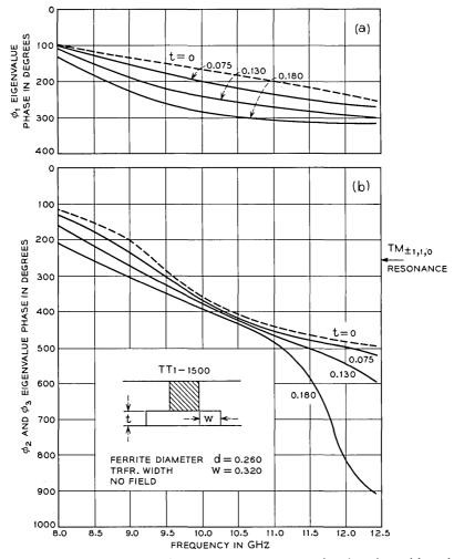
Fig. 20—The eigenvalue-phase frequency response of a junction with a full height ferrite post and different height transformers. The results show (a) the curvature in  $\angle \phi_1$  as the transformer height is increased and (b) the linearization of  $\angle \phi_2$  and  $\angle \phi_3$  in the vicinity of the TM<sub>±1,1,0</sub> resonance.
