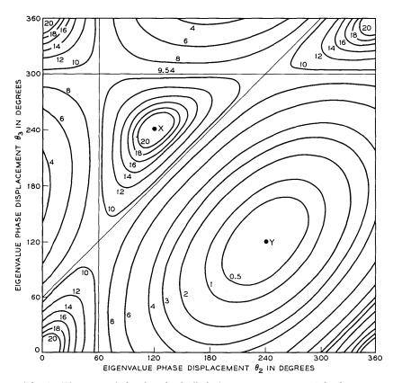
Fig. 2—The transmission loss in decibels from port 1 to port 2 is shown as a function of the phase angles between the eigenvalues. The curves are the locii of constant loss.
