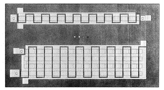
Fig. 4—Photograph of experimental bucket-brigade register chip showing an 8-bit string and a 31-bit string. Metal clock lines are approximately 3 mils wide.
