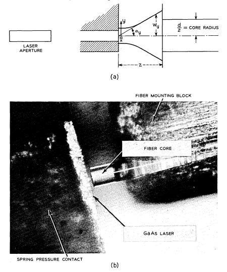
Fig. 4—(a) The Gaussian light beam emanating from a laser aperture (typical dimensions:  $1 \ \mu m \times 13 \ \mu m$ ) is injected into the core of an optical fiber. In its far field the beam diverges at an angle,  $\alpha_y$ , perpendicular to the junction plane. (b) Photograph taken through a microscope shows the 0.5-mil air gap across which light is coupled from a GaAs laser into the core of a 10-micron fiber.
