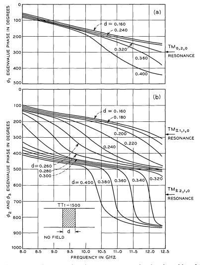
Fig. 11—The eigenvalue phase-frequency response of a junction with a full height ferrite post of various diameters. The results display (a) the lower-order  $\mathrm{TM}_{\mathfrak{s},n,\mathfrak{0}}$  modes in  $\angle \phi_1$ , (b) the lower-order  $\mathrm{TM}_{\mathfrak{s},n,\mathfrak{0}}$  modes in  $\angle \phi_2$  and  $\angle \phi_3$ .
