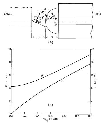
Fig. 7—(a) Cylindrical lens arrangement for collimating the laser beam perpendicular to the junction plane. (b) The radius of curvature, R, of a cylindrical lens and its axial offset, s, from the surface of a laser are plotted versus  $w_{o_3}$ , the mode width perpendicular to the junction plane. The lens is designed to collimate the beam ( $\lambda = 9000$  Å) to a 6- $\mu$ m half-width perpendicular to the junction plane.
