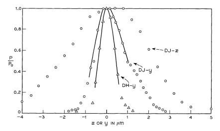
Fig. 3—Near field power distributions on the surface of junction lasers. Legend:  $\odot$  L-229 #1, DJ laser with stripe width = 6  $\mu$ m.  $\triangle$  L-363 #1, DH laser with stripe width = 13  $\mu$ m. Normalized power,  $P/P_o$ , is plotted versus distance, x, along the junction and distance, y, perpendicular to the junction.
