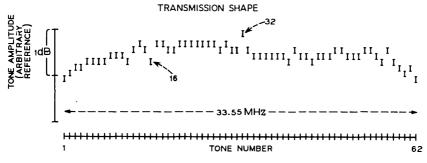
Fig. 5—Transmission shape of narrowband tone field received on horn reflector antenna.
