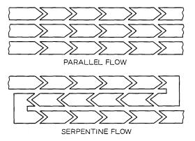
Fig. 6-Illustration of shift register layout for serpentine or parallel signal flow.
