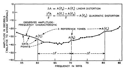
Fig. 11—Selectivity characterization of the observed amplitude-frequency characteristic.
