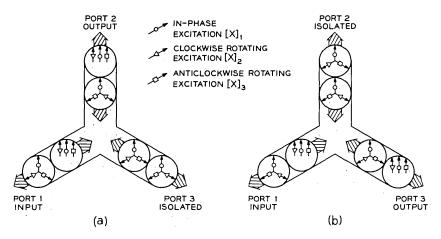
Fig. 4—A phase displacement of 120 degrees between the eigenvalues results in circulation. In (a),  $\phi_2$  is phase retarded and  $\phi_3$  phase advanced for clockwise circulation. In (b),  $\phi_2$  is phase advanced and  $\phi_3$  phase retarded for anticlockwise circulation.
