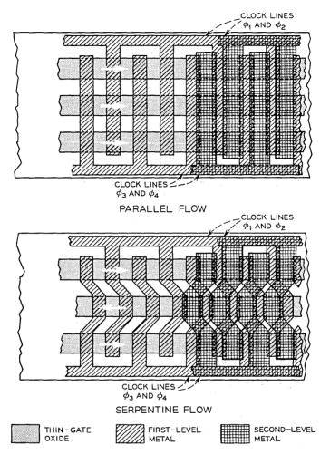
Fig. 9—Layout for serpentine and parallel flow arrays assuming a two-level metal technology for charge-coupled devices.
