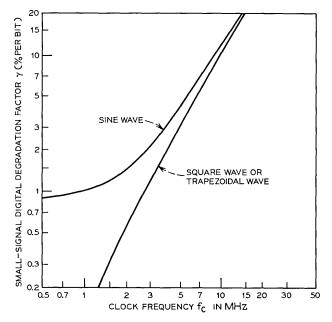
Fig. 28—Illustration of clock waveform dependence of incomplete transfer in a charge-coupled device.
