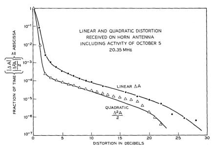
Fig. 27—Unconditional linear and quadratic distortion distributions for a bandwidth of 20.35 MHz and for the entire 1970 measurement period including the activity of October 5.
