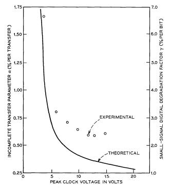
Fig. 14—Comparison of experimental and theoretical incomplete transfer parameter as a function of peak clock voltage for a bucket brigade.
