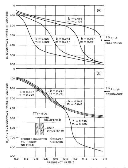
Fig. 14—The eigenvalue phase-frequency response of a junction with a full height ferrite post and containing various diameter holes and various diameter axial pins. In (a), the  $\text{TM}_{0,1,\delta}$  resonance in  $\angle \phi_1$  increases in frequency as the pin diameter is made larger. In (b),  $\angle \phi_2$  and  $\angle \phi_3$  are unaffected until the pin is sufficiently large to excite axially resonating  $\text{HE}_{\pm m,n,z}$  modes.
