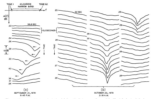
Fig. 10—Time sequential plots of selective faded amplitude-frequency characteristic. The fade depth of the lowest frequency tone (#1) is indicated when changes in amplitude occurred.
