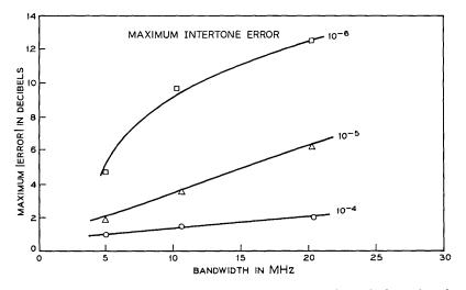
Fig. 22—A crossplot of Fig. 21 showing the observed MAX |ERROR| as a function of bandwidth for 10<sup>-4</sup>, 10<sup>-5</sup>, and 10<sup>-6</sup> fractions of the time.
