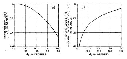
Fig. 5—(a) Transmission loss from ports 1 to 2 and (b) transmission loss from ports 1 to 3 and return loss on port 1 as a function of  $\theta_3$  with  $\theta_2$  fixed at 240 degrees.
