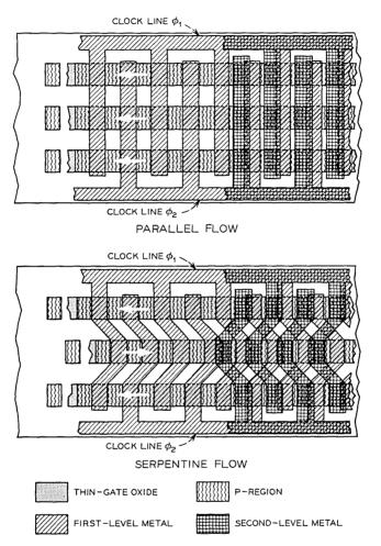
Fig. 7—Layout for serpentine and parallel flow arrays assuming a two-level metal technology for a bucket brigade.
