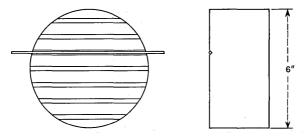
Fig. 8-Brass lap for grinding the surface of an unclad cylindrical fiber.
