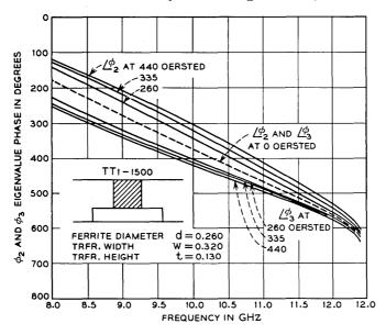
Fig. 21—The phase-frequency response of  $\phi_2$  and  $\phi_3$  for a junction with a transformer and full height ferrite post. The linearization due to the transformer permits a more even displacement of the eigenvalues with applied field.
