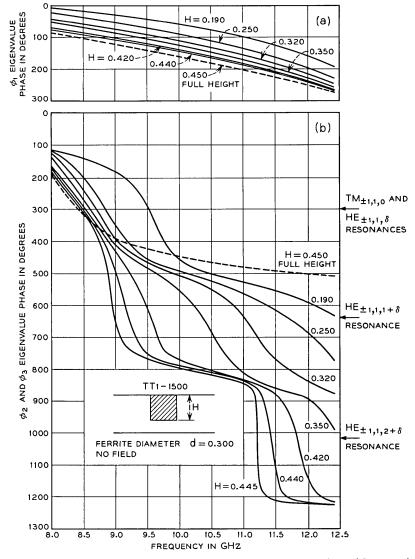
Fig. 17—The eigenvalue phase-frequency response of a junction with a partial height ferrite post. The ferrite diameter is selected to position the  $TM_{\pm 1,1,0}$  resonance at the low end of the band. The results show (a) the phase of  $\phi_1$  is only slightly changed as the ferrite height is reduced, (b) the axially resonating  $HE_{\pm m,n,z}$  modes in  $\angle \phi_2$  and  $\angle \phi_3$  increase in frequency.
