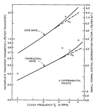
Fig. 13—Comparison of experimental and theoretical incomplete transfer parameter as a function of clock frequency for a bucket brigade.
