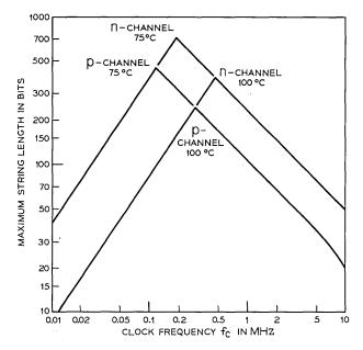
Fig. 25—Maximum length of single shift register string versus clock frequency as limited by thermal generation and incomplete transfer in a bucket brigade.
