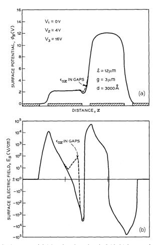
Fig. 6—Surface potential (a) and surface electric field (b) for two charge-coupled devices differing only in the presence of the dielectric in the region between electrodes.
