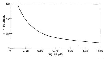
Fig. 9—The far field divergence angle,  $\alpha$ , of a Gaussian power distribution is plotted versus the half-width,  $w_o$ , of the electric field at the beam waist ( $\lambda = 9000$  Å).  $\alpha = \tan^{-1} \lambda / \sqrt{2} \pi w_0$ .
