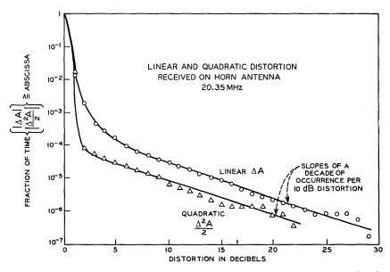
Fig. 12—Unconditional linear and quadratic distortion distributions for a bandwidth of 20.35 MHz.
