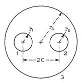
Fig. 3-Polar coordinates for the three conductors of the shielded-pair structure.
