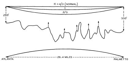
Fig. 2—Atlanta-Palmetto path profile and line-of-sight radio path for the normal (an equivalent earth radius factor k = 4/3) and the less frequent (k = 1, 2/3) atmospheric configurations. Clearance is adequate even for the extreme case of k = 2/3.
