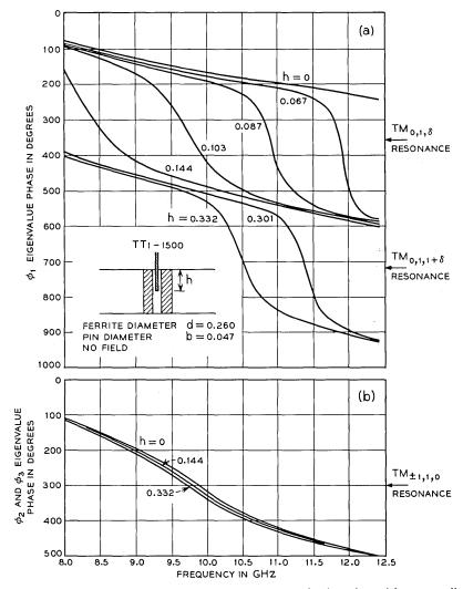
Fig. 13—The eigenvalue phase-frequency response of a junction with a centrally pinned ferrite post. The results display (a) the  $TM_{0,1,\delta}$  and  $TM_{0,1,1+\delta}$  resonances that are induced in  $\angle \phi_1$  by the variable height pin and (b) how  $\angle \phi_2$  and  $\angle \phi_3$  remain unchanged.
