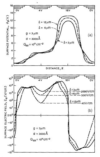
Fig. 2—Surface potential (a) and surface electric field (b) for three charge-coupled devices which differ in the electrode size but have the same gap length of 3  $\mu$ m.
