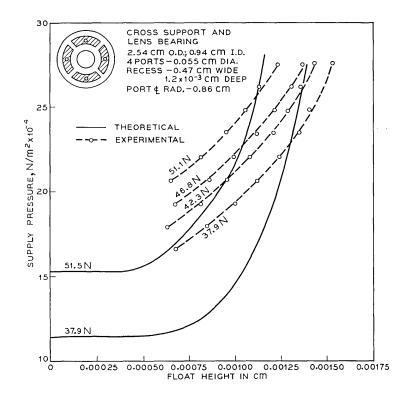
Fig. 13—Theoretical and experimental air-bearing characteristics.
