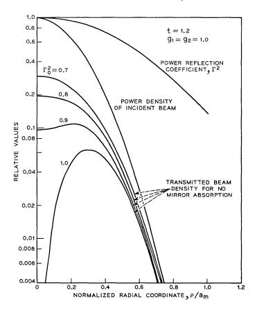
Fig. 19—Power distribution at the variable reflectivity mirror.
