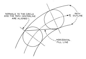
Fig. 3—Construction of a path.
