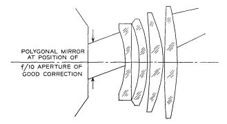
Fig. 2—Cross section of pattern generator lens.
