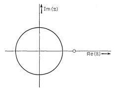
Fig. 5-Pole location of first-order projecting filter.
