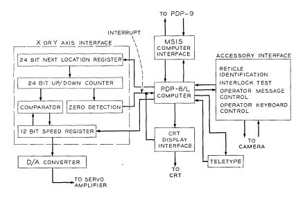
Fig. 18-Block diagram of computer/camera interface.
