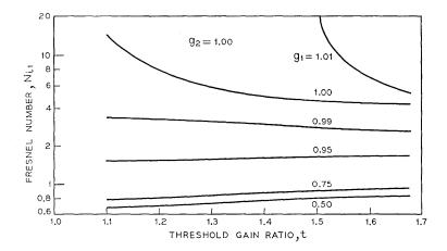
Fig. 4—Spot size of incident beam,  $N_{i1}$ .
