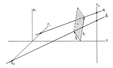
Fig. 2—An astigmatic ray pencil is defined in free space by the manifold of rays which intersect two mutually perpendicular focal lines such as  $F_1$  and  $F_2$ . At any transverse plane the intensity of the field is inversely proportional to the square root of the area defined by q and  $\hat{q}$ , the position vectors of any two rays of the ray pencil ( $\mathfrak A$  and  $\hat{\mathfrak A}$ ).
