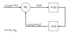
Fig. 1-PLL block diagram.
