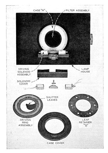
Fig. 8—Shutter assembly and components.
