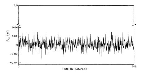
Fig. 2—Autocorrelation function of noise generator with L=13.
