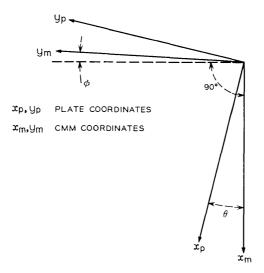
Fig. 4—CMM and plate coordinate systems.
