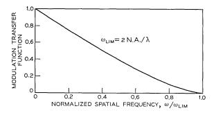
Fig. 4—The modulation transfer function of an aberration-free system as a function of the normalized spatial frequency.  $\omega$  is the line frequency in cycles per millimeter, and  $\omega_{11m}$  is the high frequency limit imposed by diffraction effects, a function only of the numerical aperture (N.A.) of the lens and the wavelength of light ( $\lambda$ ).
