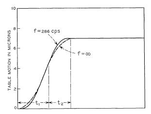
Fig. 9—Ideal rigid-body mode,  $f = \infty$ , superimposed on the actual table motion, f = 286 cps. The discrepancy between the two curves is very nearly the motion of the second mode. One notes that both modes are excited during  $t_1$  and  $t_2$ , but no motion persists in either mode once a step is completed.
