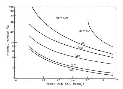
Fig. 6—Spot size of variable reflectivity mirror,  $N_m$ .
