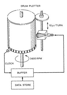
Fig. 3—Schematic of a drum plotter.
