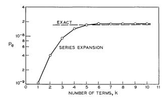
Fig. 7—Error probability versus number of terms in equation (9). Fourth-order Chebyshev pulse, 11-pulse truncation approximation; sampling instant, t=0.05 T;(S/N)=16 dB.
