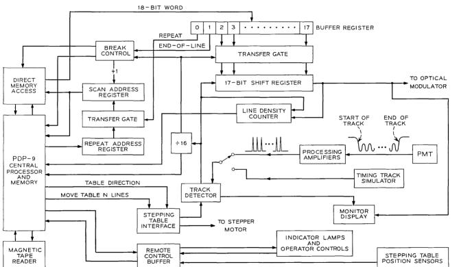
Fig. 1—Block diagram of electronics.
