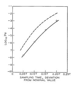
Fig. 9—Comparison of error probabilities obtained by Chernoff bound, exhaustive method, and series expansion method. Fourth-order Chebyshev pulse, (S/N) = 16 dB. [---Chernoff bound, \_\_\_\_\_\_ exhaustive method (11-pulse truncation), ooo series expansion (8-terms).]
