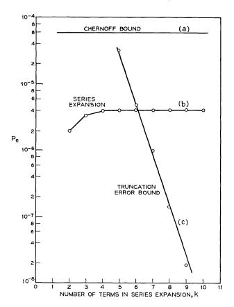
Fig. 3—Comparison of error probabilities obtained by Chernoff bound and series expansion method. (S/N)<sub>input</sub> = 14 dB; data set 203 (2400-Baud Option); 5-tap mean square equalizer; parabolic delay distortion channel (see Fig. 2).
