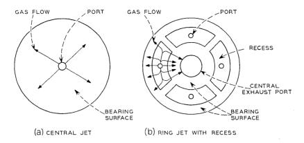
Fig. 12—Air bearing configurations.
