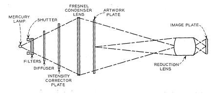
Fig. 2—Optical layout of the reduction cameras.
