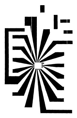
Fig. 10—Test pattern for XYMASK illustrating sloped line capability of the pattern generator.
