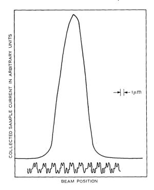
Fig. 7—Recording of calibration output. One complete cycle of the alternating signal gives four equally spaced reference marks, each of one address unit. To calibrate, number of address units between fiducial marks is held constant.
