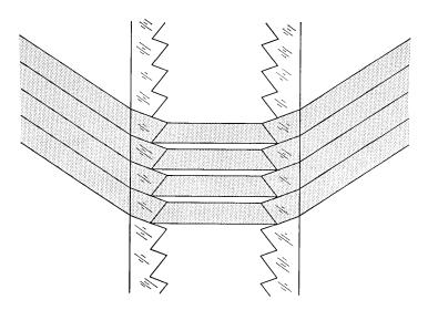
Fig. 5—Optical design of the special two-element Fresnel lens.
