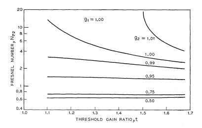
Fig. 9—Spot size of reflected beam,  $N_{r2}$ .
