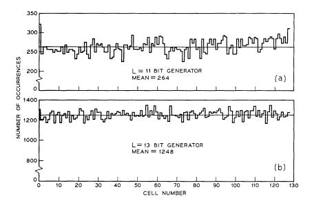
Fig. 3—Measured distribution functions for noise generators with L=11 and L=13.
