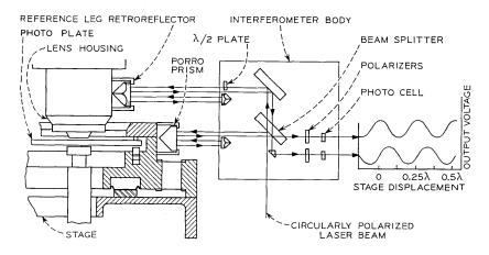
Fig. 14—Arrangement of stage position interferometer.
