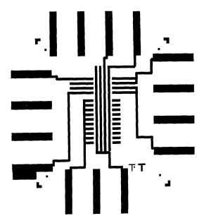
Fig. 9—Reticle produced by the electron beam.
