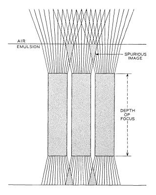
Fig. 1—Ray diagram indicating the depth of focus of a linear array of diffraction-limited spots 1  $\mu$ m apart projected into a 6- $\mu$ m emulsion of refractive index 1.56 through an ideal f/1.5 lens using 436-nm light.
