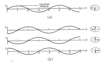
Fig. 5—Characteristics of the stepping motor. (a) 0, 1, 2,  $\cdots$ , N, are the step positions of the motor. 2, 6,  $\cdots$ , (2+4I), where I is an integer, are equilibrium positions of the motor for a particular current direction in the two-motor windings as schematically indicated by the arrows in the ellipse on the right. (b) The motor torque as a function of theta is simply translated by one step each time the current is reversed in one winding.
