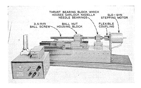
Fig. 10-Typical life-test setup.
