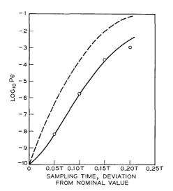
Fig. 6—Comparison of error probabilities obtained by Chernoff bound, exhaustive method, and series expansion method. Ideal band-limited signal (S/N) = 16 dB. [---Chernoff bound, \_\_\_\_\_\_ exhaustive method (11-pulse truncation), ooo series expansion (8-terms).]
