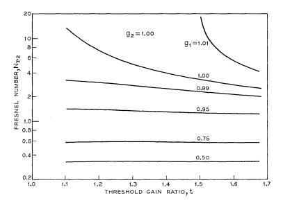
Fig. 5—Spot size of reflected beam,  $N_{r2}$ .
