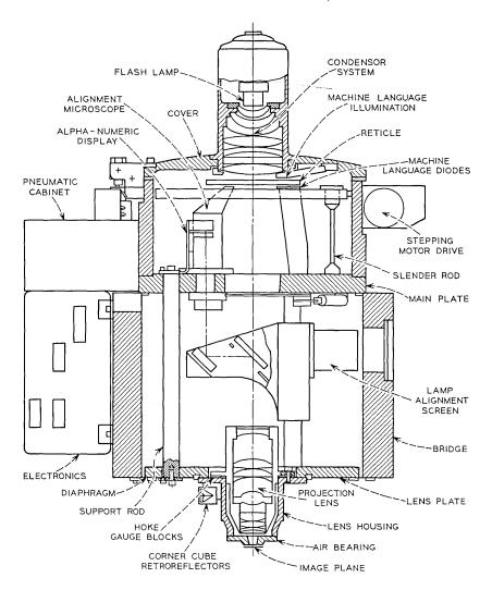
Fig. 6—Optical head assembly.
