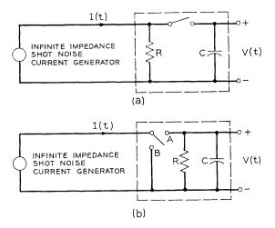
Fig. 1—RC circuits with periodically operating switch.
