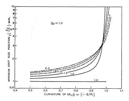
Fig. 13—Location of the minimum spot size.
