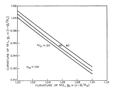
Fig. 18—Relation between mirror curvature parameters  $g_1$  and  $g_2$  and Fresnel number  $N_{i_1}$  of spot size at M1.
