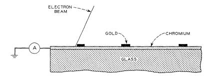
Fig. 6—Diagram of the calibration target.
