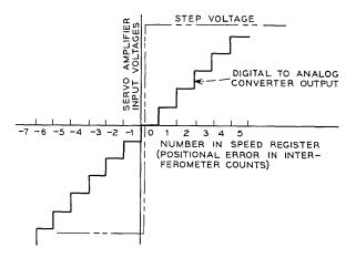
Fig. 17—Servo amplifier input voltages versus stage-positional error.
