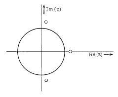
Fig. 4—Pole locations of third-order projecting filter.
