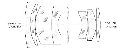
Fig. 4—Cross section of 3.5X reduction camera lens.
