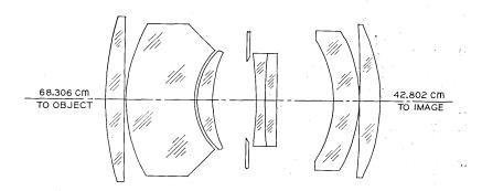
Fig. 7—Cross section of 1.4X reduction-camera lens.
