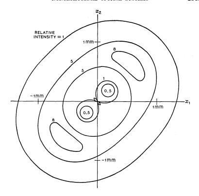
Fig. 5—This figure represents the constant intensity curves of the  $\text{TEM}_{\infty}$  mode in a nonorthogonal cavity incorporating a 6m radius mirror with an incidence angle of 30° and an image rotation of 20°. The optical axis path length is 1m, and the wavelength is  $1\mu m$ .
