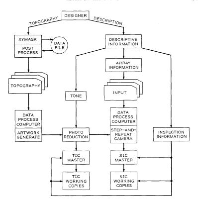
Fig. 1—Schematic of the mask-making process.
