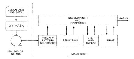
Fig. 5—Trace of a typical mask as it flows through MSIS.
