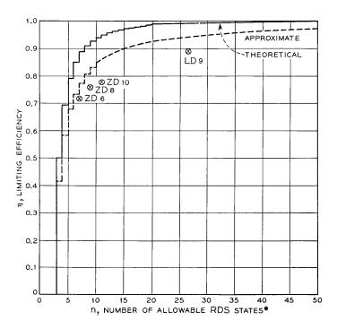
Fig. 1—Limiting efficiency vs allowable states binary alphabet (+1, -1).  $*n = M^+ - M^- + 1$ , where  $M^+$  and  $M^-$  are the upper and lower bound of the RDS.
