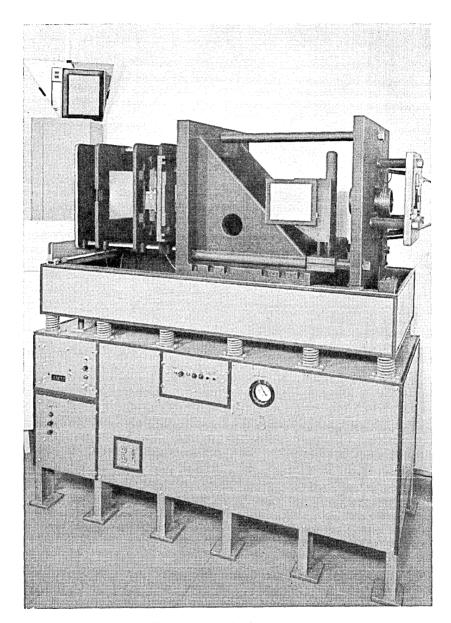
Fig. 2—3.5X reduction camera,
