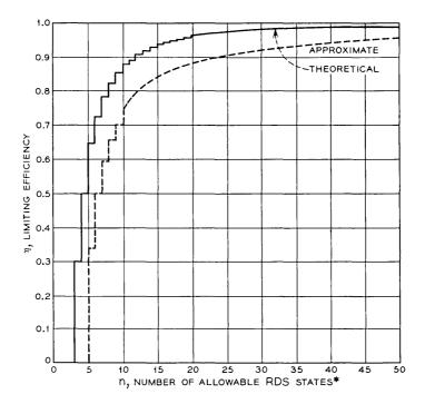
Fig. 2—Limiting efficiency vs allowable states quarternary alphabet (+3, +1, -1, -3). \* $n = M^+ - M^- + 1$ , where  $M^+$  and  $M^-$  are the upper and lower bound of RDS.
