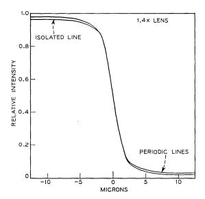
Fig. 9—Intensity distributions for isolated and periodic lines imaged by the  $1.4\mathrm{X}$  lens.
