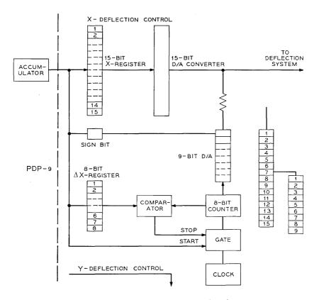
Fig. 3—Block diagram of computer interface.
