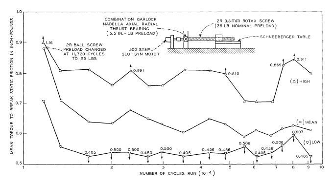
Fig. 11—Mean torque-to-break static friction versus cycles run on 2R life-test setup. Note: 1. Distance traveled per cycle = 19"; 2. Time per cycle = 190 s.
