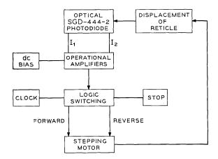
Fig. 8—Block diagram of reticle alignment electronics.
