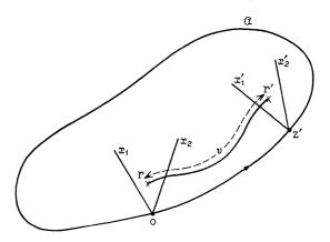
Fig. 1—Optical axis of a ring type resonator. v denotes the point characteristic of the system included between two transverse planes, z = 0 and z = z'.
