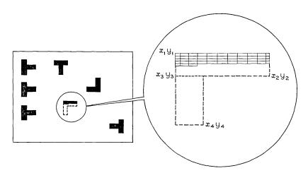
Fig. 2-Method of filling blocks using line segments.
