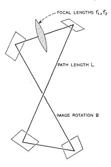
Fig. 4—A cavity with image rotation is represented. It incorporates a lens and four plane mirrors which define a nonplanar path. As a result of the twist of the path, this resonator is nonorthogonal. When the lens is astigmatic, the resonating modes do not exhibit the same patterns as in the case of more conventional cavities.
