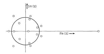
Fig. 1—Locations of zeros of the spectral density function of an eighth-order process. The eighth-order projecting filter has poles at the zero locations that are outside the unit circle.
