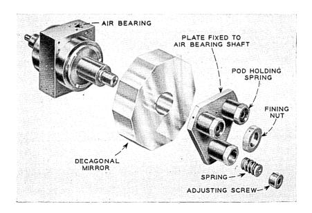
Fig. 4—Telescopic view of the decagonal mirror adjustment.
