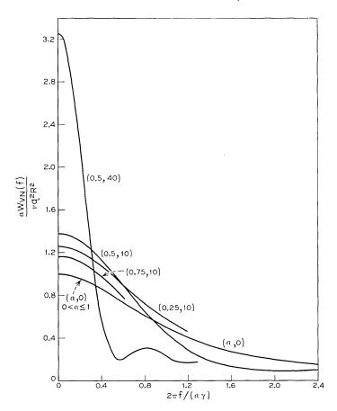
Fig. 3—Power spectrum of V(t) in Fig. 1a.  $W_{V_N}(f) = \text{2-sided power spectrum of } V(t) \text{ minus } DC \text{ spike due to } V_{dc} = \nu \ qR.$   $I(t) = \sum_k q \delta(t - t_k), \ \nu = \text{Arrival Rate, } \gamma = 1/(RC);$   $\alpha = \text{Fraction of time switch is closed; }$  T = Length of switch cycle;  $(\alpha, \gamma T) = \text{Curve parameters. }$
