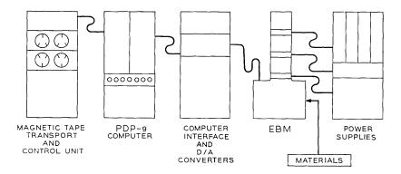
Fig. 1-Block diagram of the equipment.
