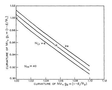
Fig. 17—Relation between mirror curvature parameters  $g_1$  and  $g_2$  and Fresnel number  $N_{i1}$  of spot size at M1.
