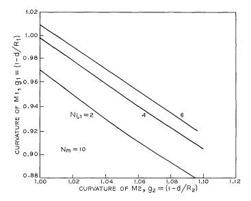
Fig. 15—Relation between mirror curvature parameters  $g_1$  and  $g_2$  and Fresnel number  $N_{41}$  of spot size at M1.
