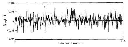
Fig. 4—Cross-correlation function of noise generators with L=11 and L=13.
