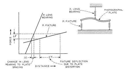
Fig. 9—Theoretical prediction of focus control system performance.
