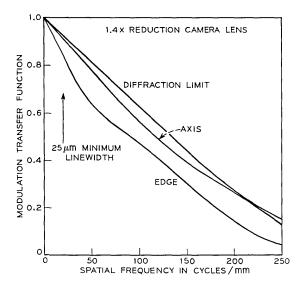
Fig. 8-MTF curves for the 1.4X reduction-camera lens.
