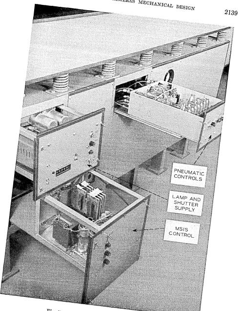
Fig. 7—Pneumatic and electrical controls.
