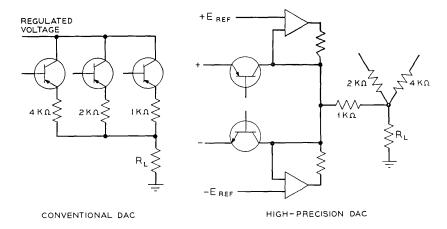
Fig. 4—Simplified diagram of conventional and high-precision DACs.
