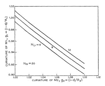
Fig. 16—Relation between mirror curvature parameters  $g_1$  and  $g_2$  and Fresnel number  $N_{41}$  of spot size at M1.
