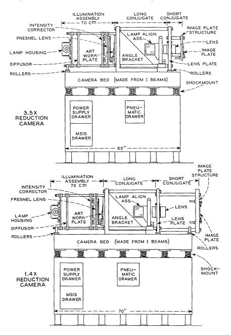
Fig. 1—Schematic of 3.5X and 1.4X reduction cameras.
