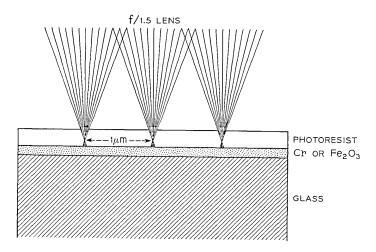
Fig. 3—Ray diagram of projected point sources spaced at 1- $\mu$ m intervals in 0.3- $\mu$ m-thick photoresist coating on 0.1- $\mu$ m-thick film of metal or semitransparent mask material (f/1.5 lens, 436-nm light).
