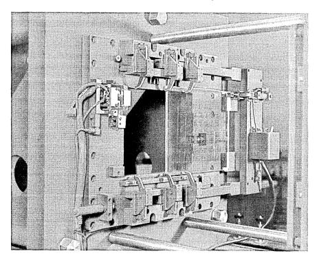
Fig. 6—Insertion mechanism for artwork.
