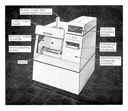
Fig. 2—The step-and-repeat camera.
