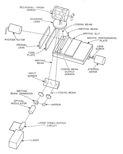
Fig. 1-Schematic of primary pattern generator.
