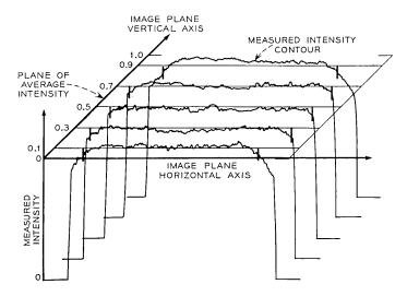
Fig. 4—Measured intensity distribution in the image plane. The maximum deviations of the measured intensity contours from the plane of average intensity are  $\pm$  7 percent.
