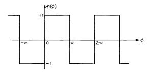
Fig. 2—Phase comparator characteristic.
