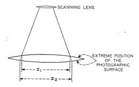
Fig. 2—The effect of photographic plate camber.
