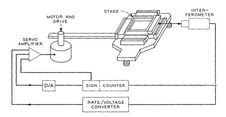
Fig. 16—Block diagram of stage-positioning servo system.
