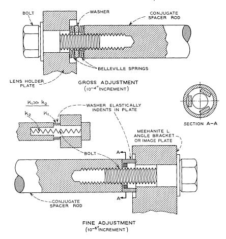
Fig. 5—Adjustment mechanism for conjugates of reduction camera.
