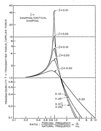
Fig. 4—Transmissibility versus frequency for a single-degree-of-freedom rigid-body system.
