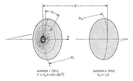
Fig. 1—Nonsymmetrical resonator.
