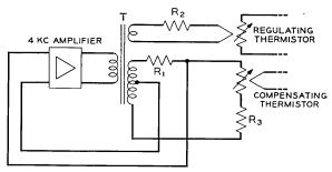
Fig. 29 — Ambient temperature compensation oscillator.
