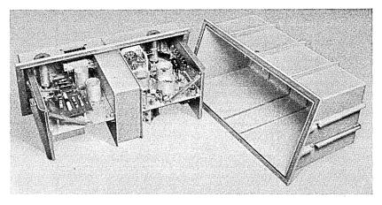
Fig. 3 — Line amplifier and housing.
