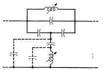
Fig. 11 — Schematic of a delay equalizer section, (dotted capacitors are parasitic).
