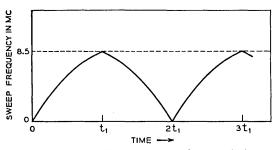
Fig. 15 — Method of scanning the system gain characteristic to convert cosines of frequency into cosines of time.
