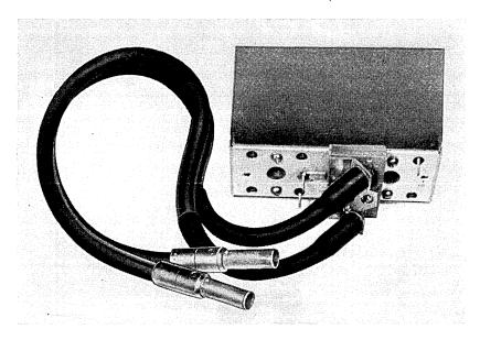
Fig. 13 — Fixture for delay equalizer section adjustment.
