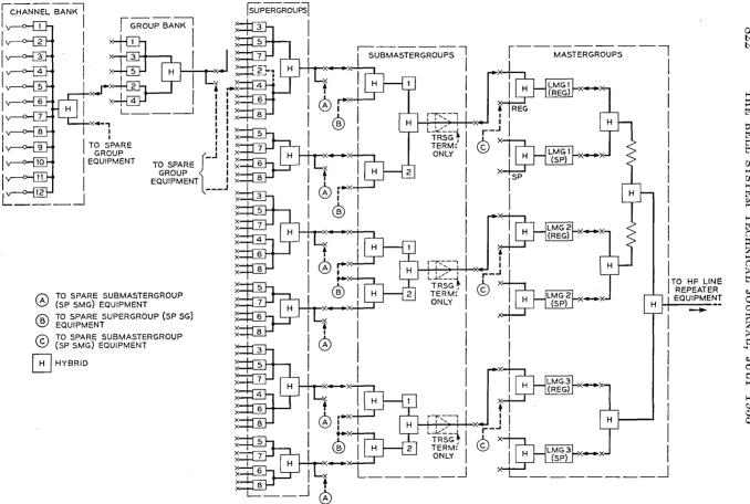
Fig. 19 — Terminal transmission equipment for an all-message system.
