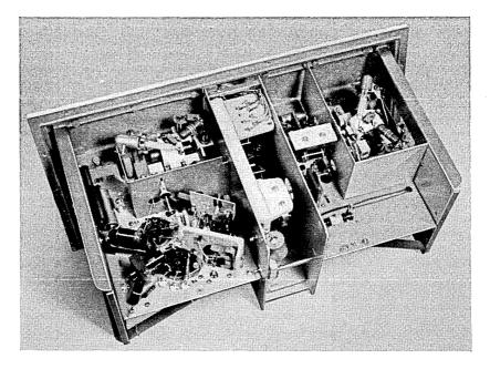
Fig. 4 — Line amplifier, wiring side.
