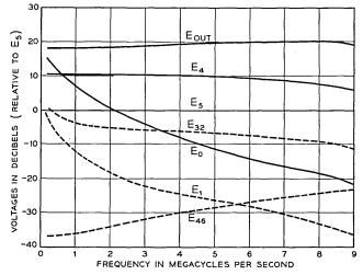
Fig. 18 — Relative levels of signal voltages in line amplifier referred to voltage at grid of lower triode. Thermistor at mid-range value.
