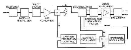
Fig. 19 - L3 receiving terminal block diagram.
