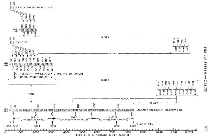
Fig. 20 — Frequency translations in the terminal for an all-message system.
