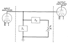
Fig. 11(a) — Regulating network block schematic.
