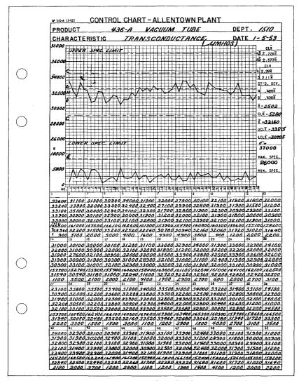
Fig. 5 — A typical control chart (436A vacuum tube).
