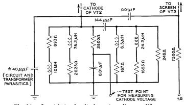
Fig. 14 — Input beta circuit elements — line amplifier.
