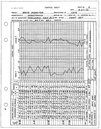
Fig. 4 — A typical control chart (1507E inductor).
