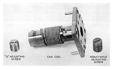
Fig. 12 — Inductor with adjusting screws.
