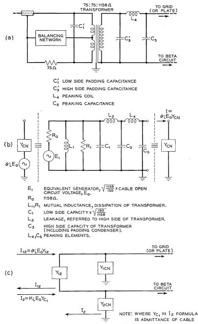
Fig. 8 — Coupling Network Circuits. (a) Physical elements. (b) On-ground equivalent circuit, adequate for gain and feedback computations in an amplifier configuration employing on-ground coupling networks. (c) Off-ground equivalent Circuit.
