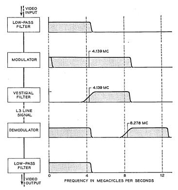
Fig. 2 — Television terminal modulation processes.
