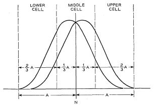
Fig. 6 — A three-cell pattern superimposed on a frequency distribution of individual units of product when the average is allowed to vary  $\pm \frac{1}{3}\sigma$ .
