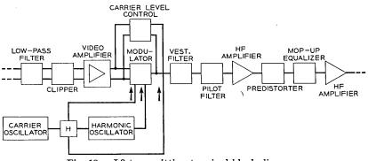
Fig. 18 — L3 transmitting terminal block diagram.
