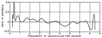
Fig. 17 — Final gain characteristic of a 100 mile L3 line after equalication with 15 cosine shapes.
