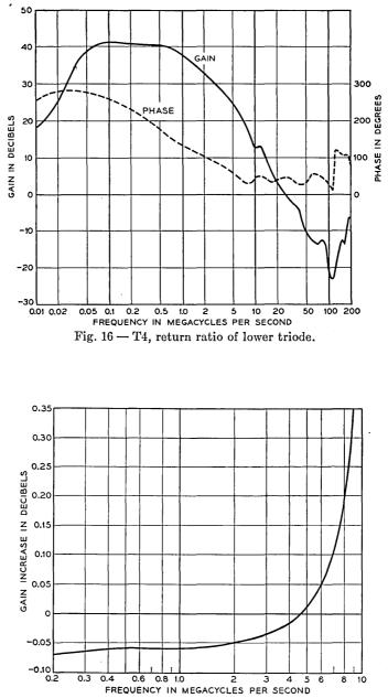
Fig. 17 — Mu beta effect, amplifier gain change for a one db decrease in each transconductance.
