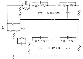
Fig. 10 — Cosine equalizer circuit (tenth harmonic) showing dissipation and range corrections.
