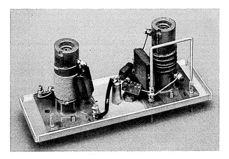
Fig. 14 — Model of a typical delay equalizer section.
