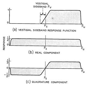
Fig. 5 — Response function of a vestigial sideband carrier system.
