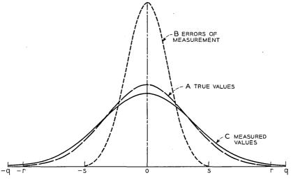
Fig. 1 — Effect of measuring errors.
