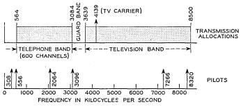
Fig. 1 — Frequency allocations for L3 combined television-telephone transmission.
