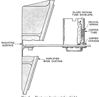
Fig. 6 — Heat conducting tube shield.
