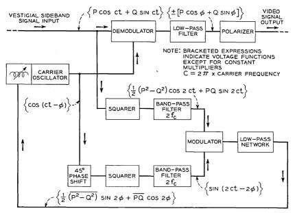
Fig. 7 — Functional diagram of the L3 homodyne demodulation process.
