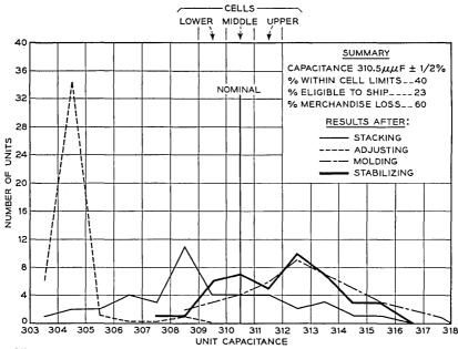
Fig. 10 — A summarized frequency distribution of a 310.5-mmf mica condenser at various stages of manufacture.
