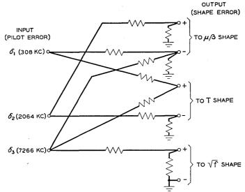
Fig. 2 — Schematic of regulation system computer.
