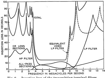
Fig. 9 — Insertion loss of the transmitting terminal filters.
