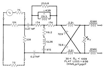
Fig. 6 — Circuit of the regulating network for repeater temperature.
