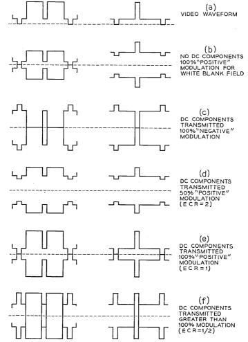
Fig. 9 - Typical television signals. Alternative carrier frequency waveforms.
