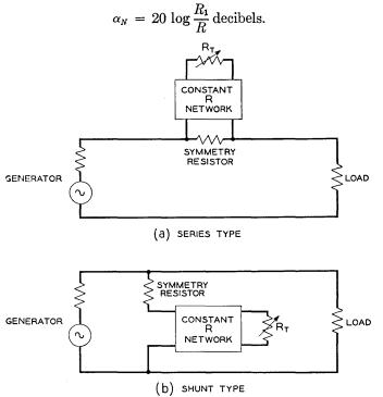
Fig. 5 — Block diagram of Bode Regulating Network.
