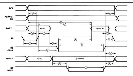
Figure 22. External I/O or Memory Read/Write Timing
