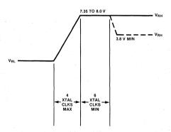
Figure 14. Z8682 RESET Pin Input Waveform
