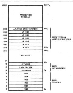
Figure 16. Z8681/82 Logical Program Memory Mapping
