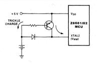
Figure 13, Recommended Driver Circuit for **Power-Down Operation**
