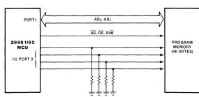
Figure 10. Port 0 Address Lines Tied to Logic 0
