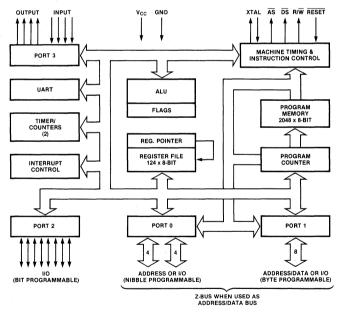
Figure 3. Functional Block Diagram
