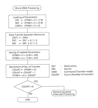
Figure 3.3 (3). Micro DMA Processing Flowchart
