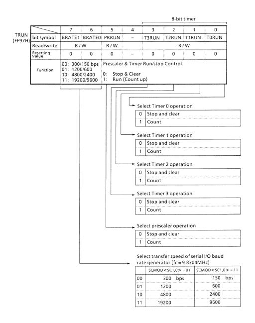
Figure 3.6 (6). Timer/Serial Channel Control Registers (TRUN)
