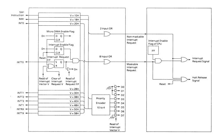
Figure 3.3 (8). Block Diagram of Interrupt Controller
