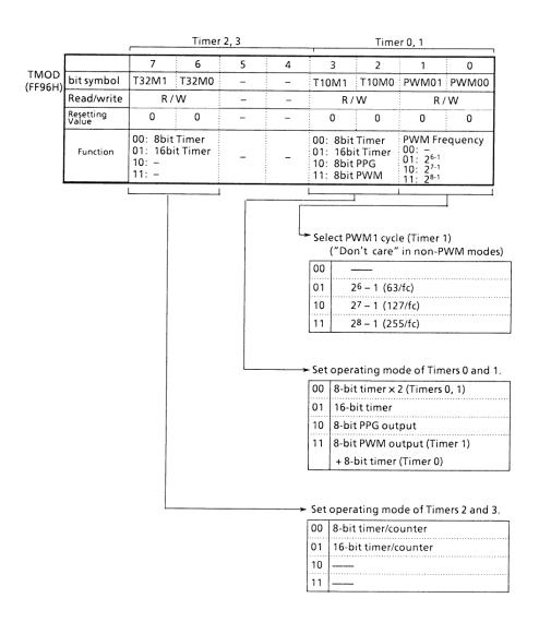
Figure 3.5 (4). 8-bit Timer Mode Register TMOD
