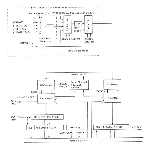
Figure 3.7 (8). Block Diagram of Serial Channel
