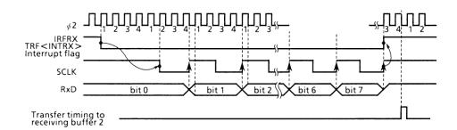
Figure 3.7 (11). Receiving Operation (I/O Interface Mode)
