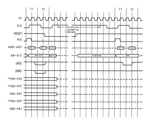
Figure 3.1 (1b). TMP90C401 Reset Timing
