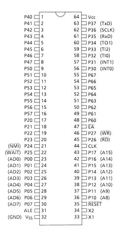
Figure 2.1 (1). Pin Assignment (Shrink Dual Inline Package)
