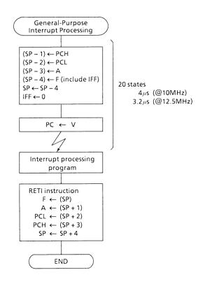
Figure 3.3 (2). General-Purpose Interrupt Processing Flowchart
