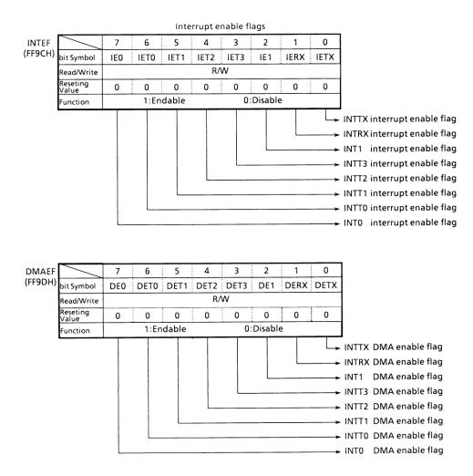
Figure 3.3 (9). Interrupt/Micro DMA Enable Flags
