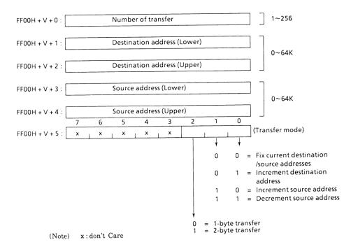
Figure 3.3 (4). Parameters for Micro DMA Processing
