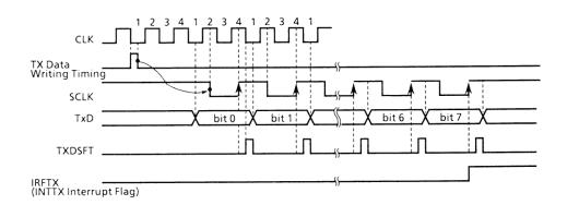
Figure 3.7 (10). Transmitting Operation (I/O Interface Mode)
