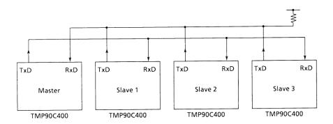
Note: for the wake-up operation, P33 should be always selected as the TxD pin of the slave controllers, and put in the open drain output mode.
