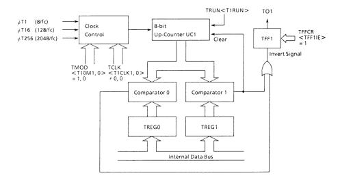
Figure 3.6 (11). Block Diagram of 8-bit PPG Mode
