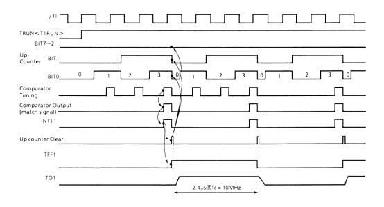
Figure 3.6 (8). Pulse Output (50% duty) Timing Chart
