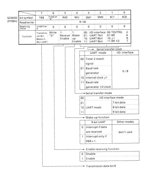
Figure 3.7 (2). Serial Channel Mode Register
