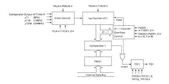
Figure 3.6 (12). Block Diagram of 8-bit PWM Mode
