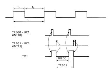
In this mode, programmable pulse is generated by the inversion of the timer output put each time the 8-bit upcounter 1 (UC1) matches the timer register TREG0 or TREG1.
