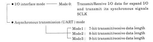
The mode 3 accommodates a wake-up function to start the slave controllers in a controller serial link (multi-controller system). Figure 3.7 (1) shows the data format (1-frame data) in each mode.
