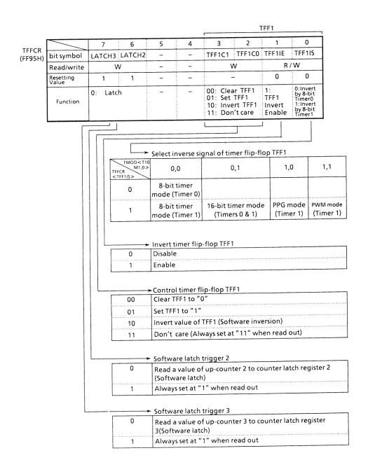
Figure 3.6 (7). 8-bit Timer Flip-Flop Control Register (TFFCR)
