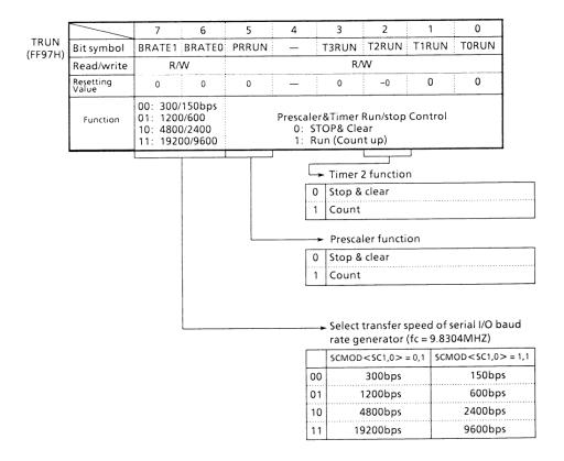
Figure 3.7 (5). Timer/Serial Channel Operation Control Register
