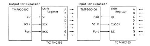
Figure 3.7 (9). I/O Interface Mode
