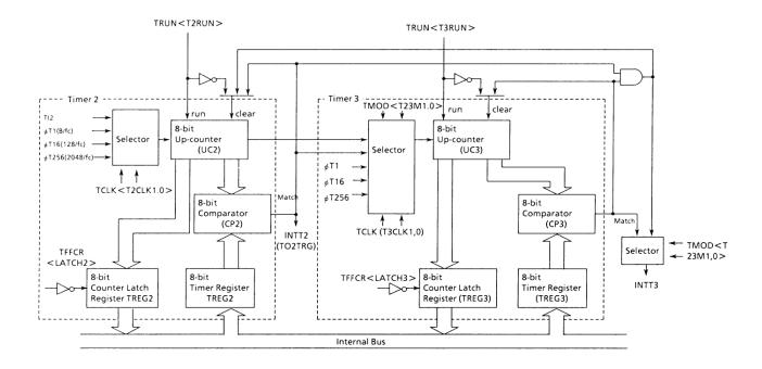
Figure 3.6 (2). Block Diagram of 8-bit Timer/Counter (Timers 2 and Timer 3)
