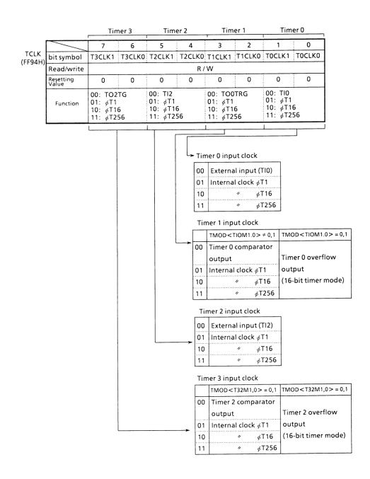
Figure 3.6 (5). 8-bit Timer Clock Control Register (TCLK)
