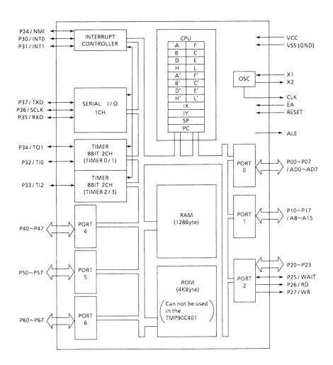
Figure 1. TMP90C400 Block Diagram
