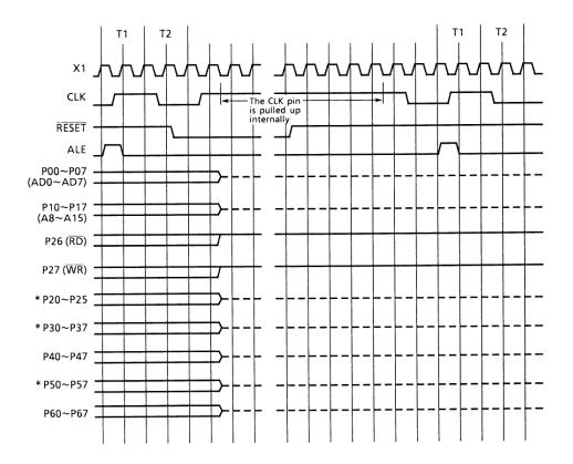
Figure 3.1 (1a). TMP90C400 Reset Timing
