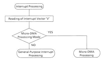
Figure 3.3 (1). Interrupt Response Flowchart
