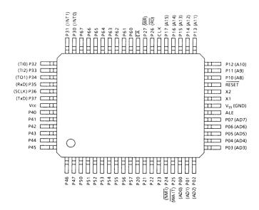
Figure 2.1 (2). Pin Assignment (Flat Package)
