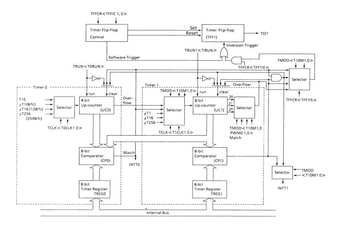
Figure 3.6 (1). Block Diagram of 8-bit Timers (Timers 0 and 1)
