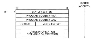
Figure 4.6 TMP68010 Stack Frame
