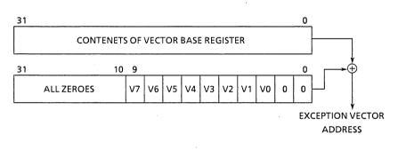
Figure 4.4 Exception Vector Address Calculation (TMP68010)
