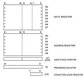
Figure 1.1 User Programmer's Model (TMP68000/TMP68008/TMP68010)
