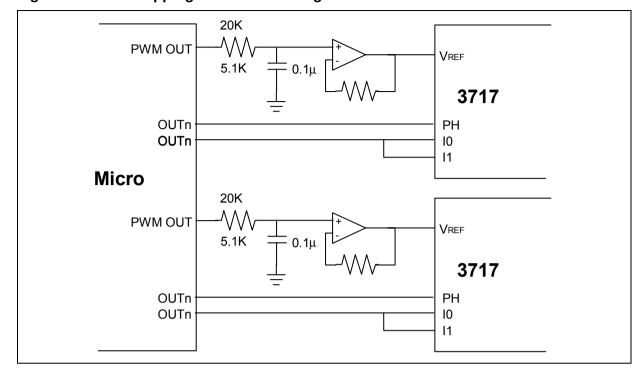
Figure 14. Microstepping connection using PBL3717
