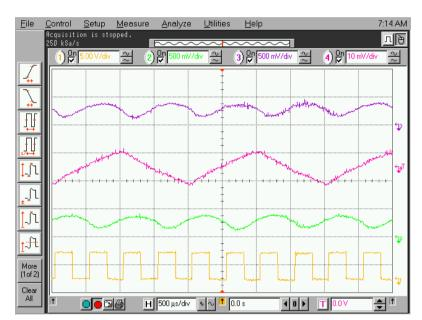
Figure 8. Waveforms when motor has stalled
