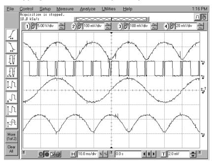
Figure 12. Microstepping waveforms with improved performance at zero current.
