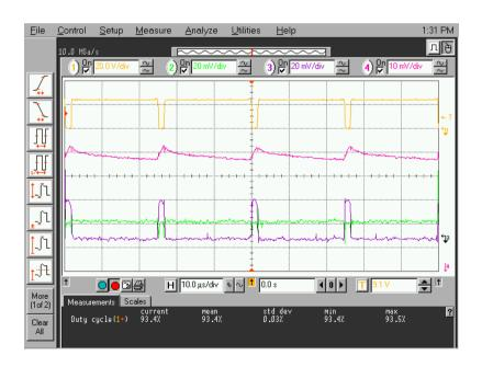
At the start of each cycle the bridge is turned on and the motor current flows through the sense resistor to produce the voltage  $V_{sense}$ . However at this operating point the sense voltage is already greater than the Vref input voltage, as can be seen in Figure 10. The comparator will detect that  $V_{sense}$  is greater than Vref and cause the circuit switch the bridge into the recirculation mode and
