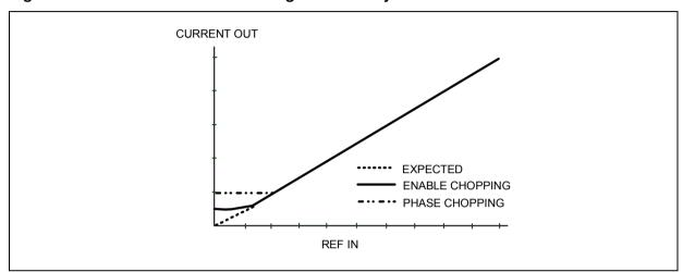
Figure 11. Transfer function showing nonlinearity
