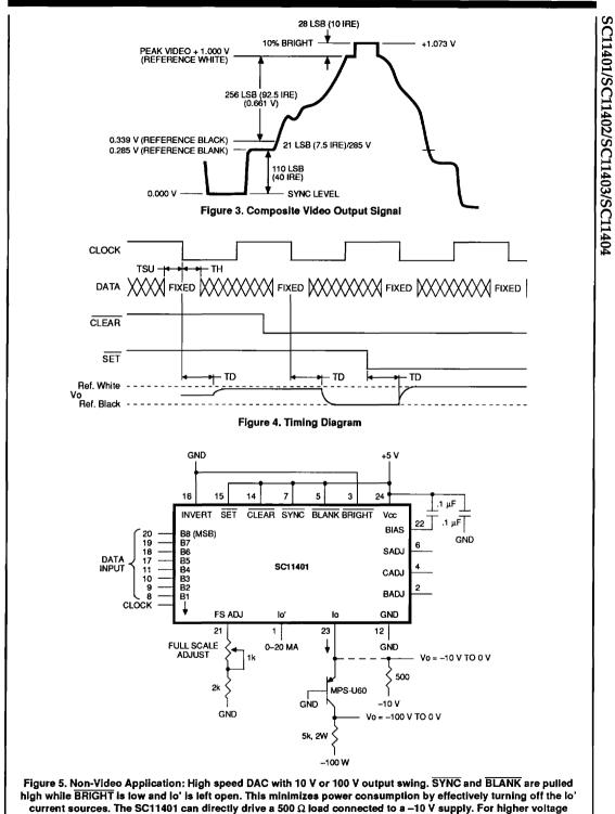
swings, a high voltage PNP transistor, such as the MPS-U60 can be used, along with a 5K, 2  $\Omega$  resistor. 637
