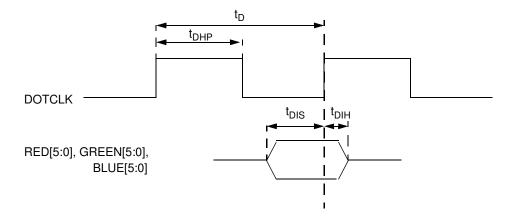
Figure 5-2. Pixel Port Interface Signals
