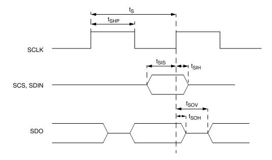
Figure 5-3. Serial Interface Signals
