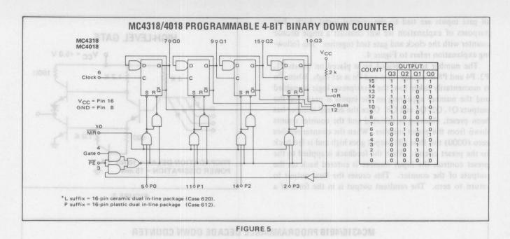
Comparisons of MC4016 (Decade Counter – Figure 4) and MC4018 (Binary Counter – Figure 5)
