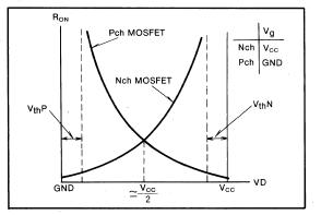
Fig.14 MOS switch turn-on resistance
