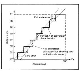
Fig.11 Zero and full scale error
