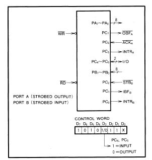
Fig. 7 Mode 1 port A and port B I/O example
