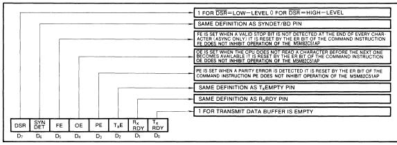
Fig. 10 Status information  $(C/\overline{D}=1, \overline{RD}=0)$
