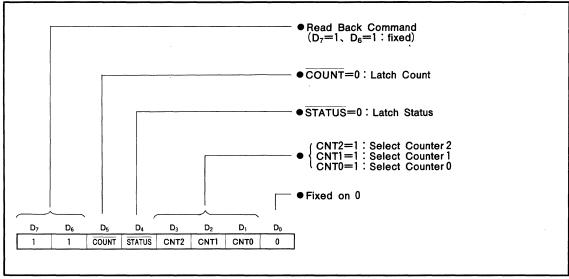
Fig. 7 Read Back Command Format
