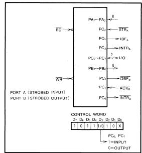
Fig. 8 Mode 1 port A and port B I/O example
