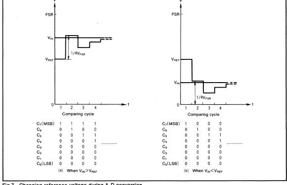
Fig.7 Changing reference voltage during A-D conversion
