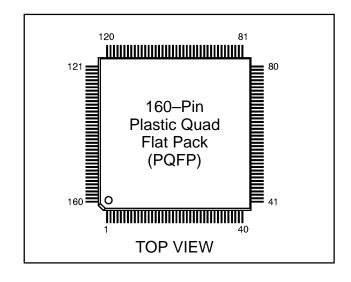
Figure A. Pin Configuration
