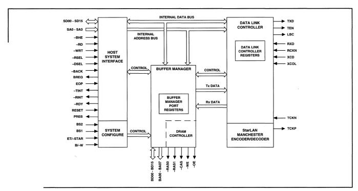
**EtherStar Ethernet Controller Block Diagram**
