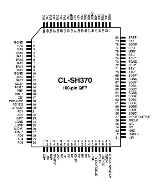
100-pin Quad Flat Pack (QFP) Pin Diagram
