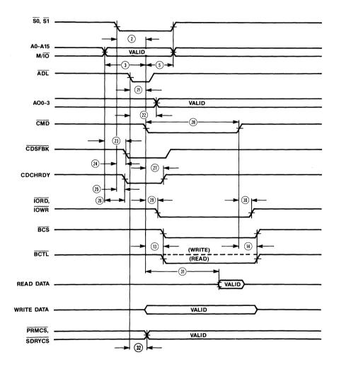
**Synchronous Extended Cycle Timing**
