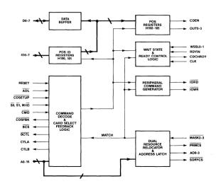
Figure 1. 82C575 Functional Block Diagram
