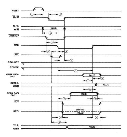
**POS Register Setup Cycle Timing**
