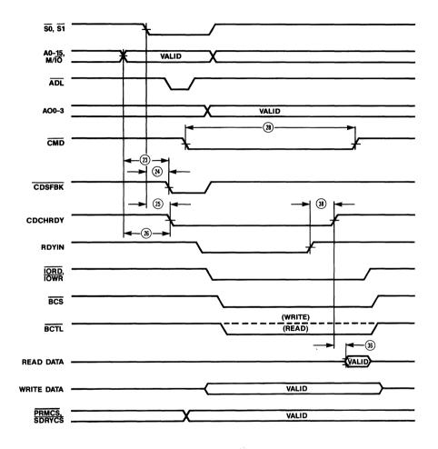
**External Asynchronous Extended Cycle Timing**
