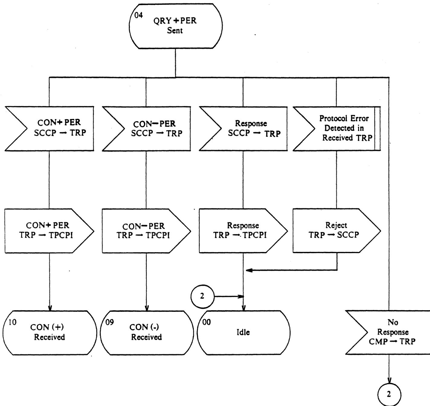
Figure 7/Q.774. Transaction Portion (Sheet 3 of 10)
