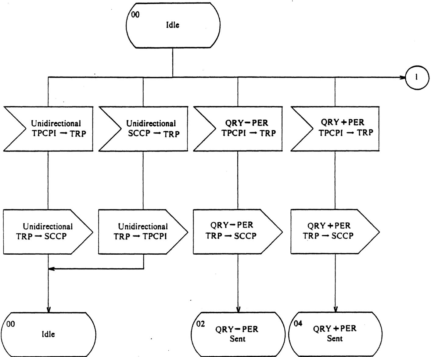
Figure 7/Q.774. Transaction Portion (Sheet 1 of 10)
