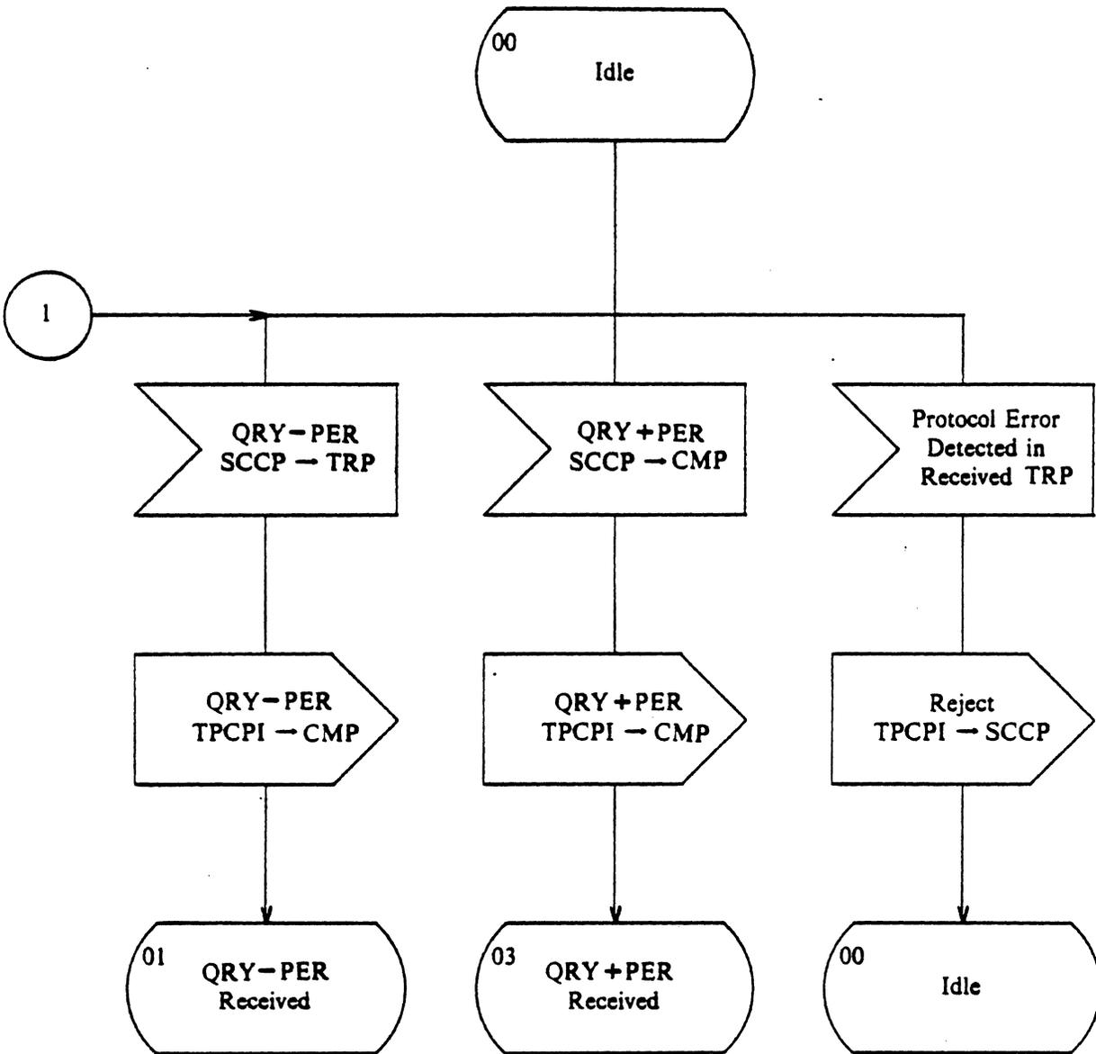
Figure 7/Q.774. Transaction Portion (Sheet 2 of 10)
